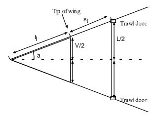
and the lengths of the bridles (s) and the trawl wings (t) are known. The wingspread V is then calculated as:
