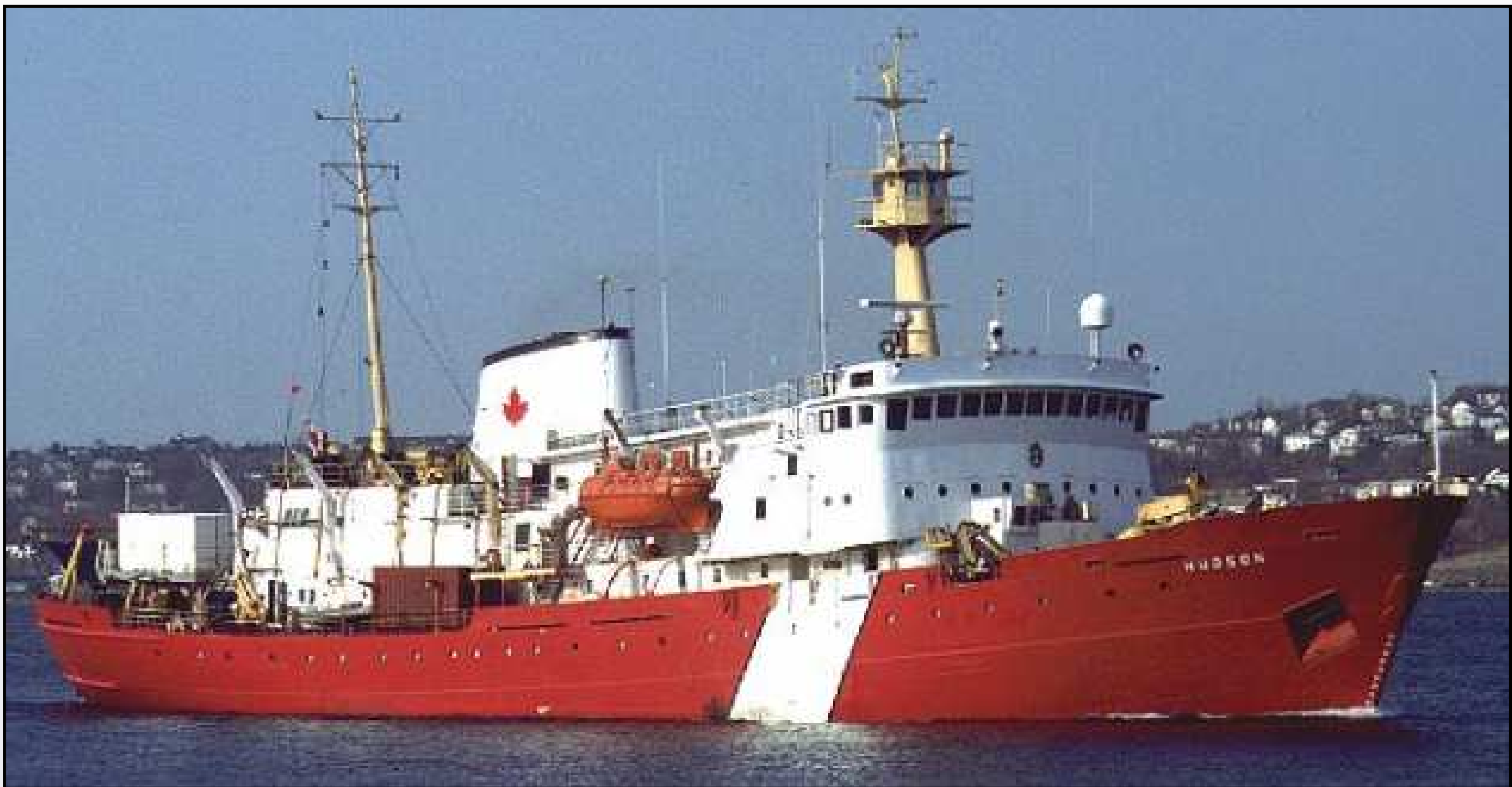
CCGS Hudson - Canada's most famous scientific ship. Commissioned in 1964 and still making important scientific contributions after 47 years on the high seas. CCGS Hudson is 90.4 m in length with 3740 gross tonnage. She is owned and operated by the Canadian Coast Guard and carries 60 berths, with 28 of those available to scientists. There are three laboratories, one fore and aft and one below deck as well as chart rooms and computer banks off the bridge. CCGS Hudson has been the mainstay of the oceanographic research programs on the east coast of Canada.
