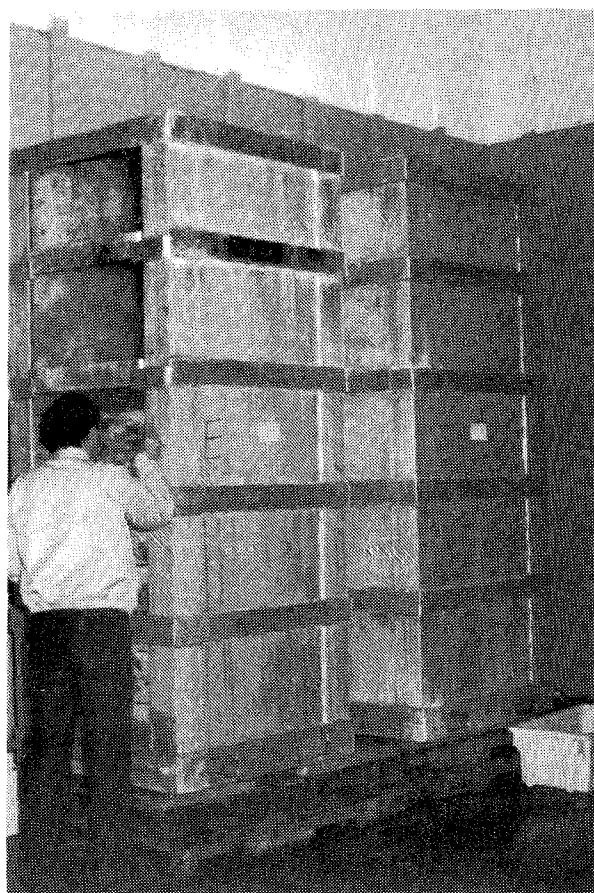
(iv) Pallet E during curing phase, pallet dimensions 1 m x 1 m x 2.5 m.
