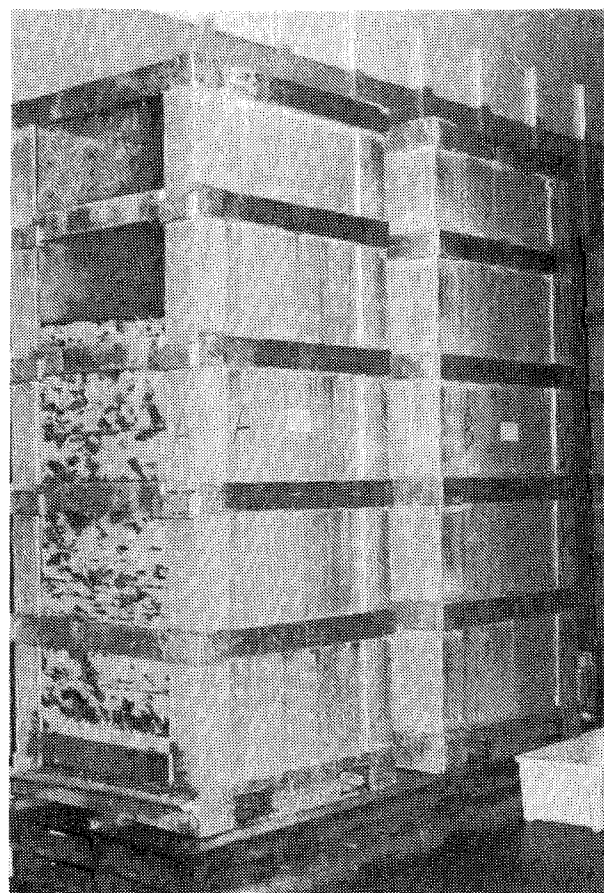
(iii) Pallet A during curing phase (note the division of daily levels).
