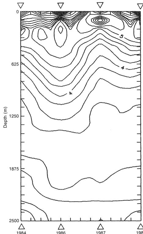
Fig. 14. Isopleths of temperature at station 4 of the Frederikshaab Section during 1984, 1986, 1987 and 1988.
