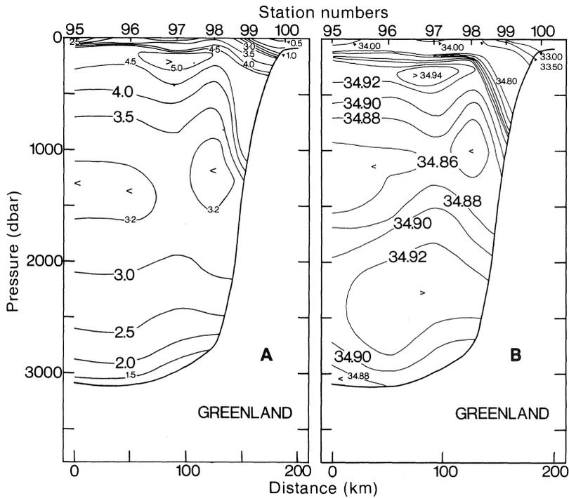
Fig. 5. (A) potential temperature, and (B) salinity along the Frederikshaab Section, 2 November 1984.
