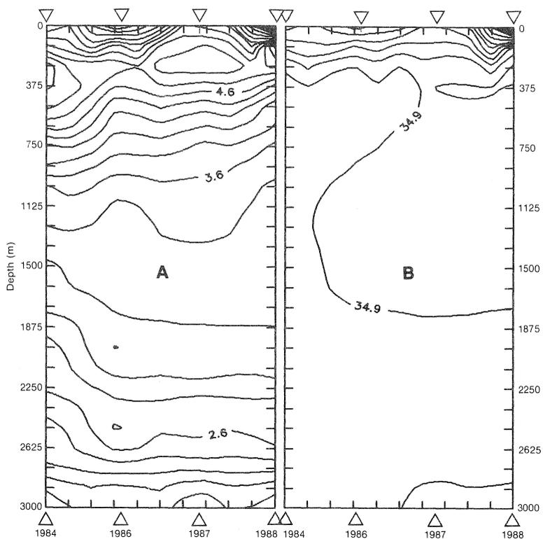
Fig. 12. Isopleths of (A) temperature, and (B) salinity at station 3 of the Cape Desolation Section during 1984, 1986, 1987 and 1988.
