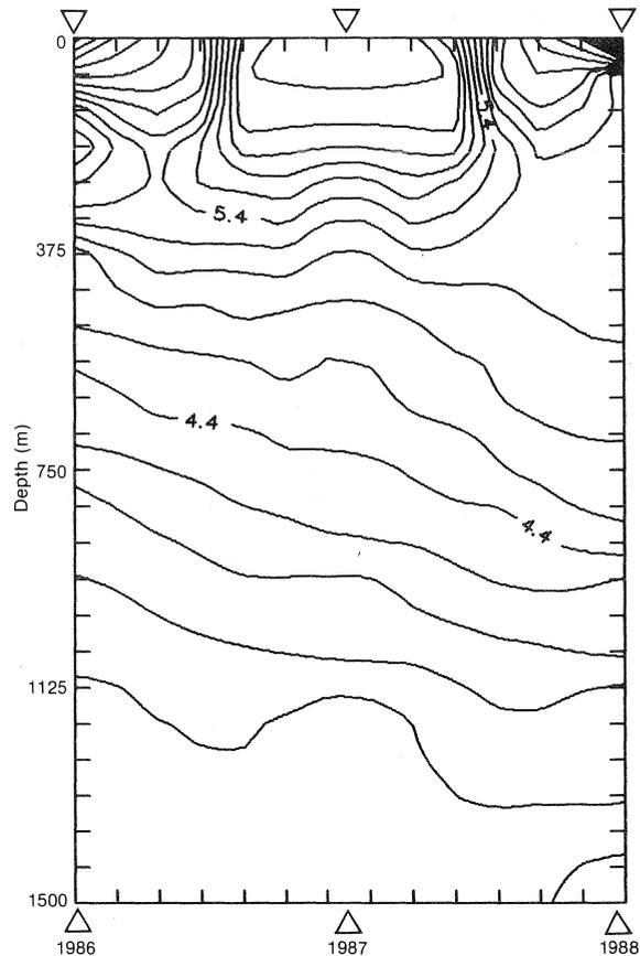
Fig. 9. Isoleths of temperature at station 3 of the Cape Farewell Section during the period 1986–88.
