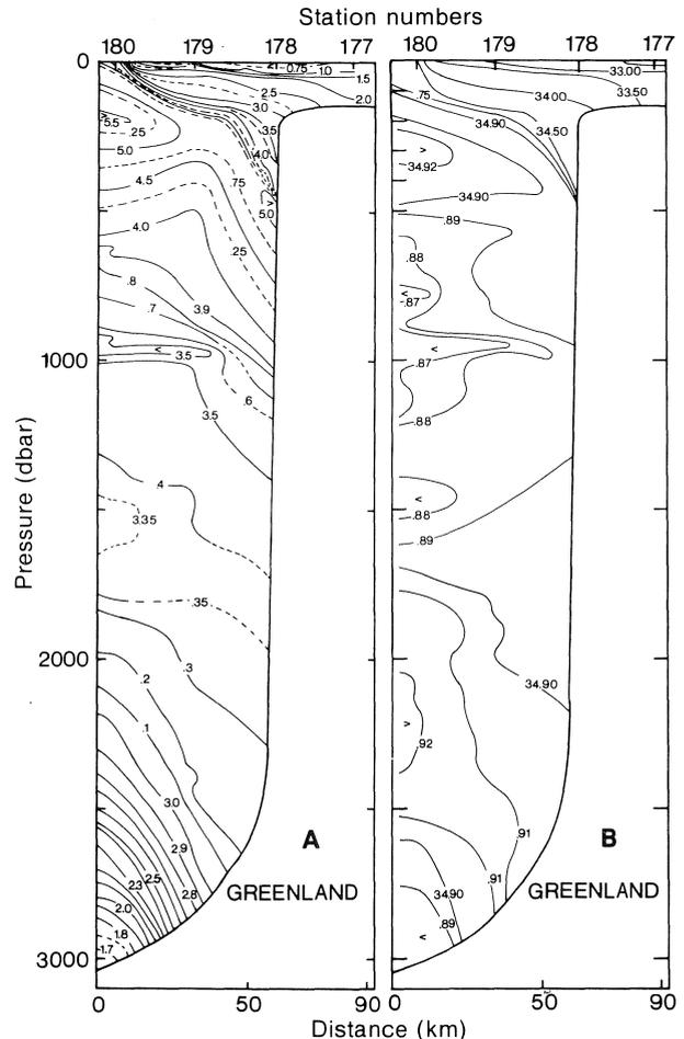
Fig. 7. (A) potential temperature, and (B) salinity along the Cape Desolation Section, 12 November 1987.
