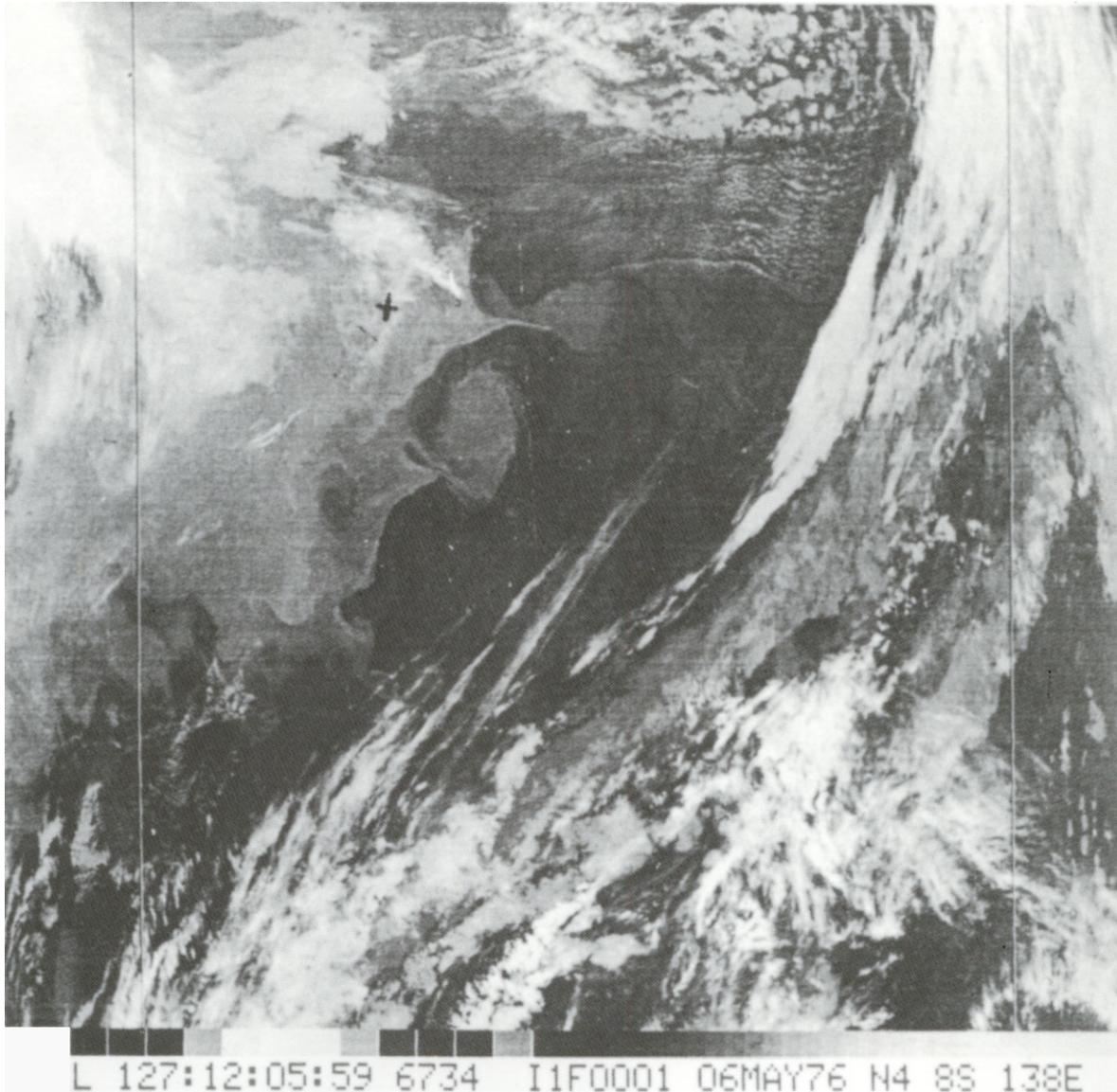
Fig. 21. NOAA Very High Resolution Radiometer (VHRR) satellite imagery of the area 46°–49°N, 43°–47°W for 6 May 1976; location of Flemish Cap is indicated by "+"; mesoscale structures of cold (gray) and warm (black) water masses are visible east and southeast of Flemish Cap (from Trites, MS 1977).
