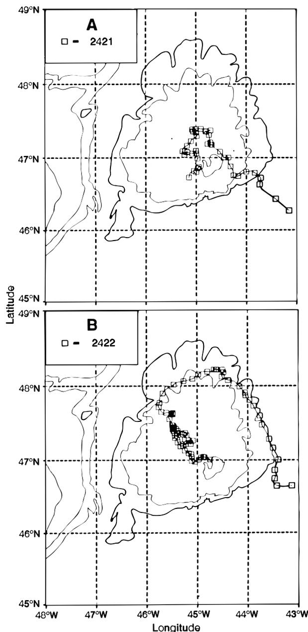
Fig. 8. Drift track of buoys (A) 2421, first point at 46.72°N, 45.16°W at 1800z day 14, last point at 1800z day 54, symbol every 24 hours; (B) 2422, first point at 46.99°N, 44.50°W at 1800y day 77, last point at 0600y day 148, symbol every 24 hours (from Ross, 1981).
