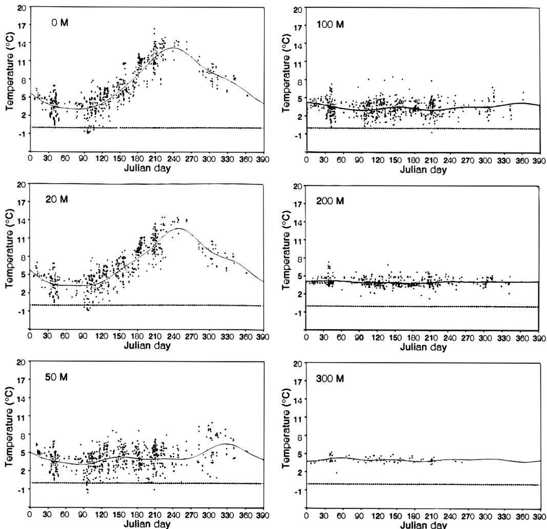
Fig. 17. Temperature values for all years at depths of 0, 20, 50, 100, 200 and 300 m for area FC1 in Fig. 2, together with the fitted regression curves (from Colbourne, MS 1993).
