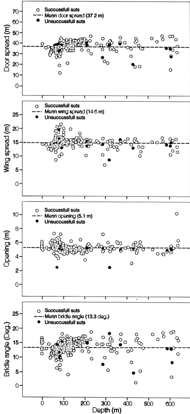
Fig. 4. Relationship of *W. Templeman* (old doors) door spread, wing spread, opening and bridle angles with depth.
