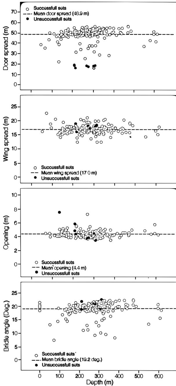
Fig. 5. Relationship of *W. Templeman* (new doors) door spread, wing spread, opening and bridle angle with depth.
