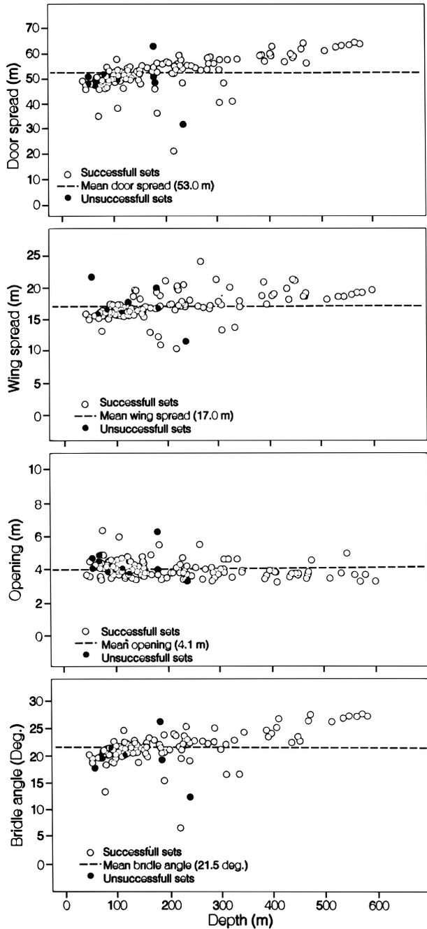
Fig. 7. Relationship of *Teleost* door spread, wing spread, opening and bridle angle for depths to 1 200 m.
