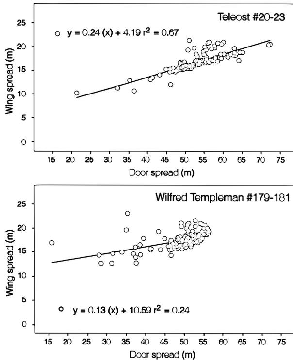
Fig. 3. Relationship between wing spread and door spread for the *Teleost* and *W. Templeman* survey trawls.
