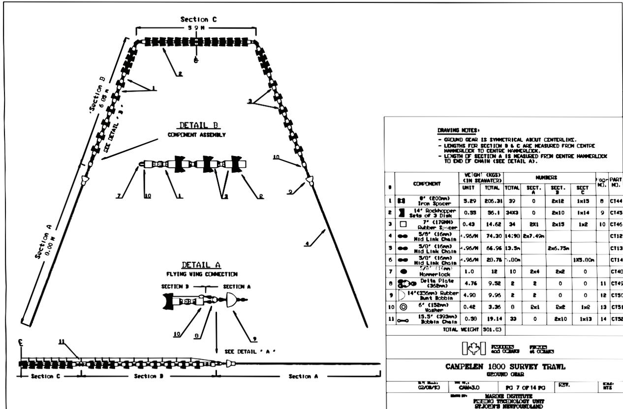
Fig. 2. Footgear details of the Campelen 1800 survey trawl.
