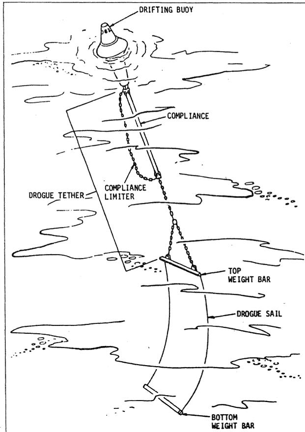
Fig. 1. Schematic diagram of a drogued drifting buoy.
