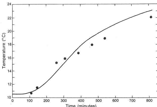
Fig. 3. Central temperature equilibration of a 50-cm egg mass in 25°C water following a change from the initial 10.5°C water. (The curve represents theoretical temperature changes for a sphere with a thermal diffusivity of 0.0036 cm<sup>2</sup>/sec.)
