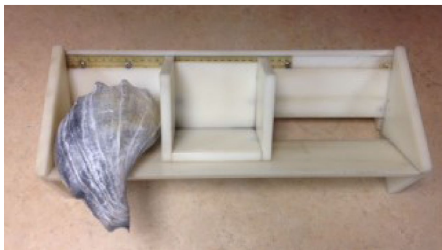
Figure 88. An example of how to obtain width measurements using the Whelk Sampling board.
