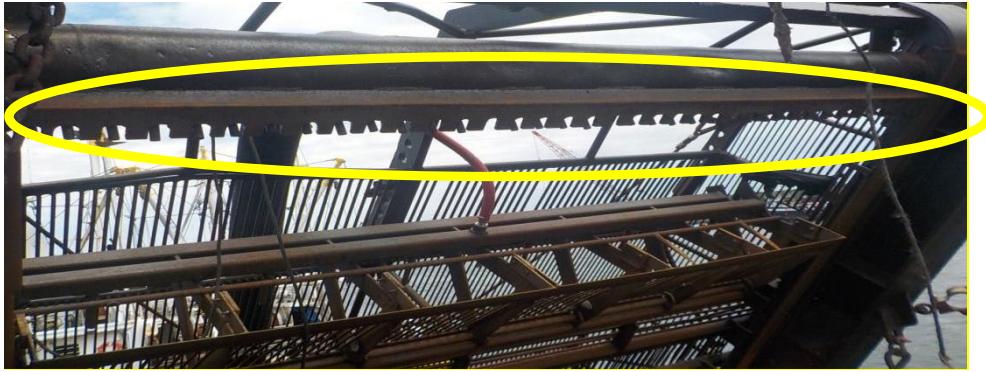
Figure 46. Example of nozzles on the manifold section of a clam/quahog dredge.
