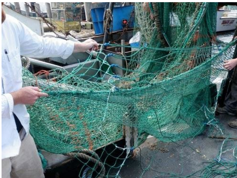
Figure 32. A large mesh belly panel installed in a bottom trawl.
