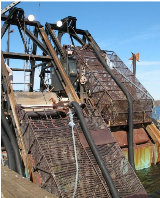
Figure 47. Example of a tow line attached to a dredge.
