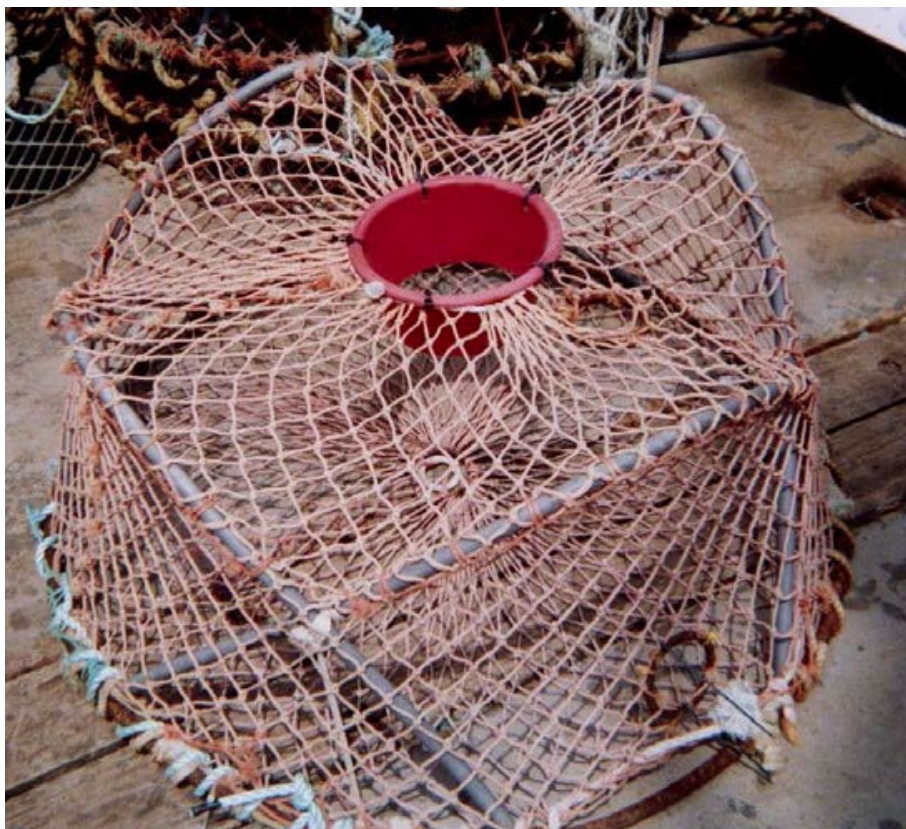
Figure 12. Red crab trap. Note entrance ring (red, top) and escape vent (brown, lower right-hand corner).
