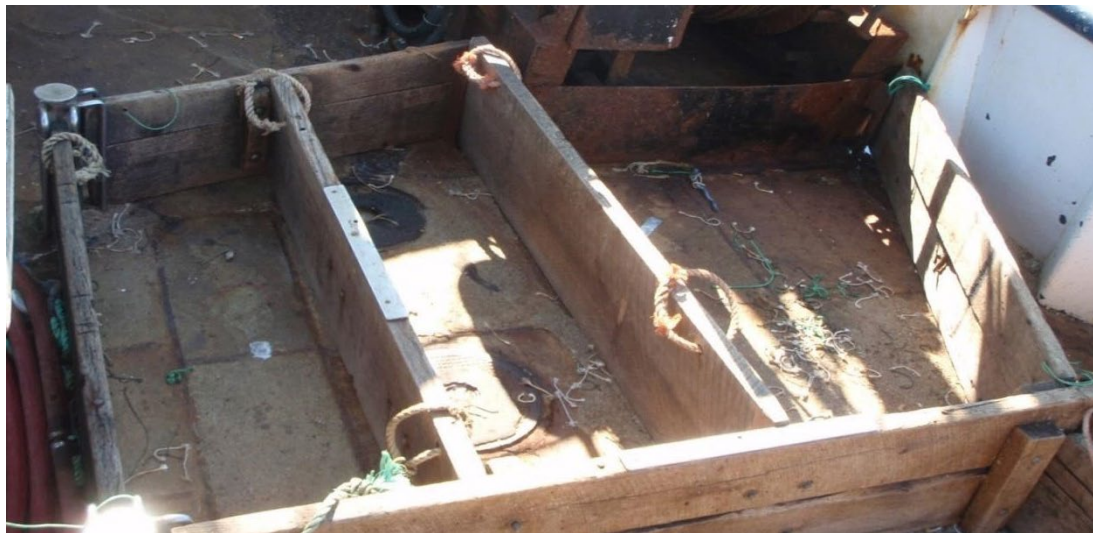
Figure 71. An example of multiple checker pen shapes present on deck. Note the ropes attached to each board, which allow the fishermen to manipulate the size and shape of the checker pen, as needed.
