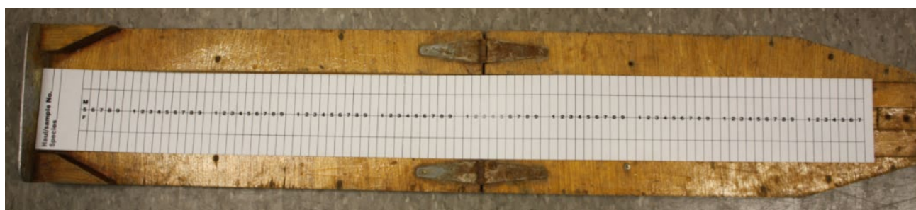
Figure 76. An example of the finfish Length Frequency Board and Length Frequency strip being used in conjunction with each other.
