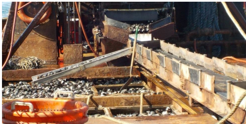
Figure 52. An example of a conveyor system set up to fill a specific section of cages on deck.
