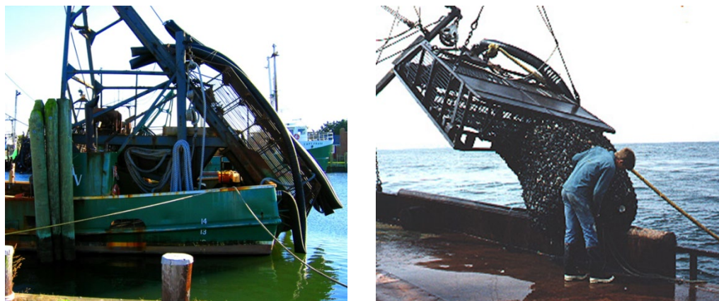
Figure 51. An example of a one-piece (left) and two-piece (right) dredge.
