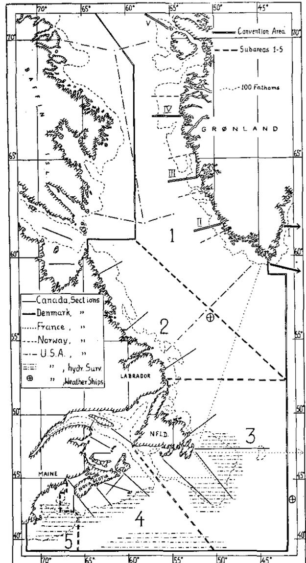
Fig. 1. Routine hydrographic work in the Convention Area. Most of the sections shown are repeated, at least, yearly. Of the sections passing the right frame of the figure the northernmost one (I) reaches Iceland, that from Cape Farvel and that from Newfoundland reach the English Channel.
