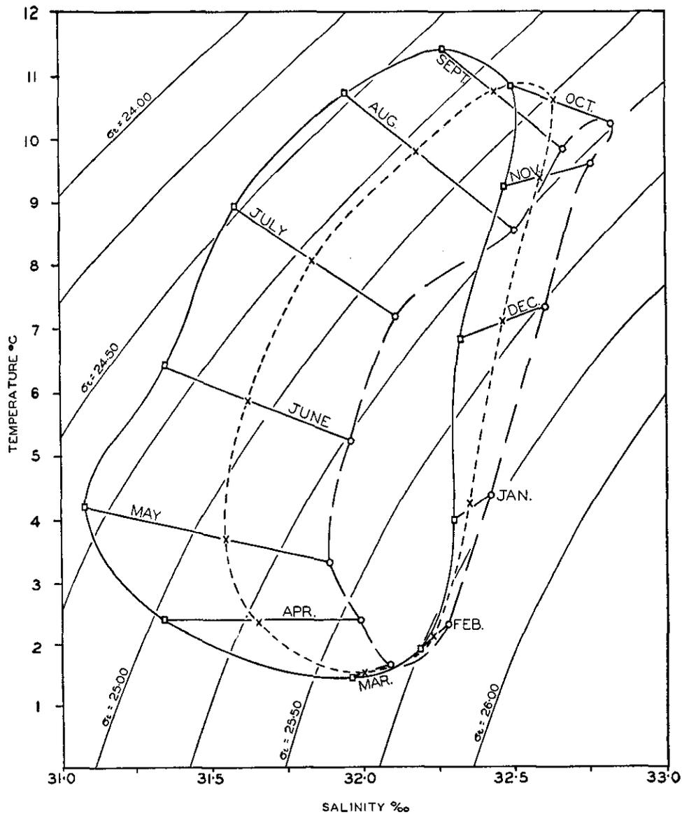
Fig. 24. Normal T-S curves for each month, and the normal annual T-S cycle for the surface——, intermediate - - - - -, and bottom — · — · — layers, Station 5 (Bay of Fundy).
