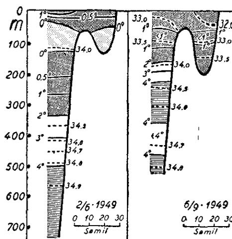
Fig. 17A. Temperature and salinity in sections across Fylla Bank in a "cold" year, 2 June and 6 Sept., 1949.
