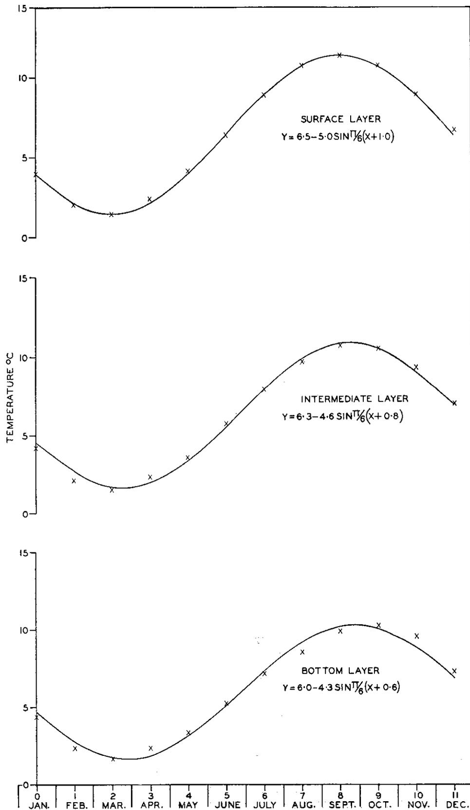
Fig. 23. Normal theoretical temperature-time curves for the surface, intermediate, and bottom layers at Station 5 (Bay of Fundy).
