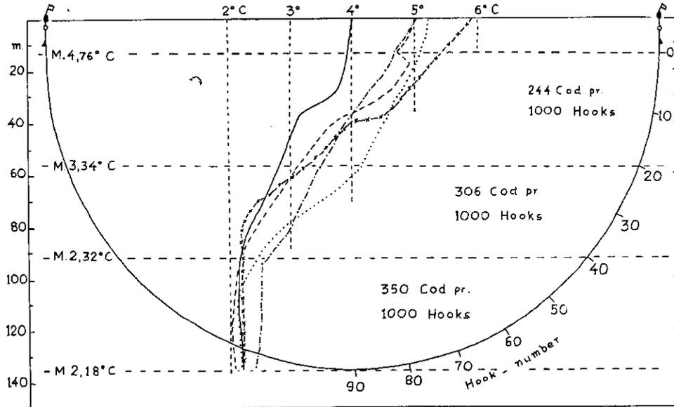
Fig. 3. Schematic drawing of a pelagic long line with temperatures and catch of cod indicated for various depths. From experiments carried out 30 July-5 August, 1953.
