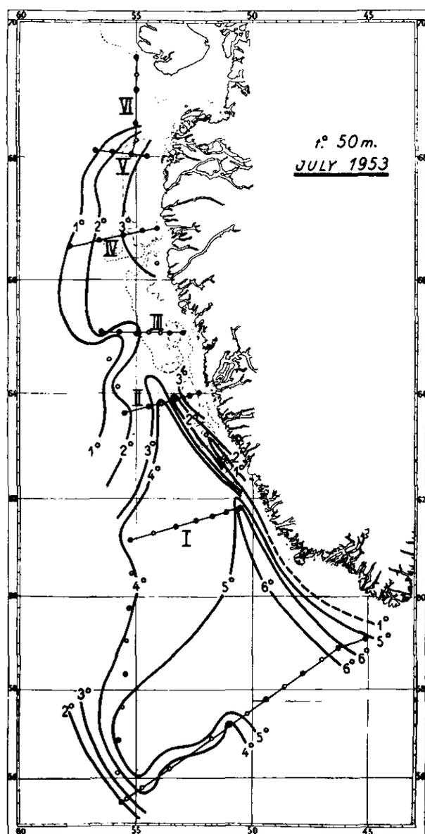
Fig. 5. Location of hydrographic sections I-VI and curves showing distribution of temperature in 50 m. depth. Open circles indicate bathythermograph stations, solid circles regular hydrographic stations.
