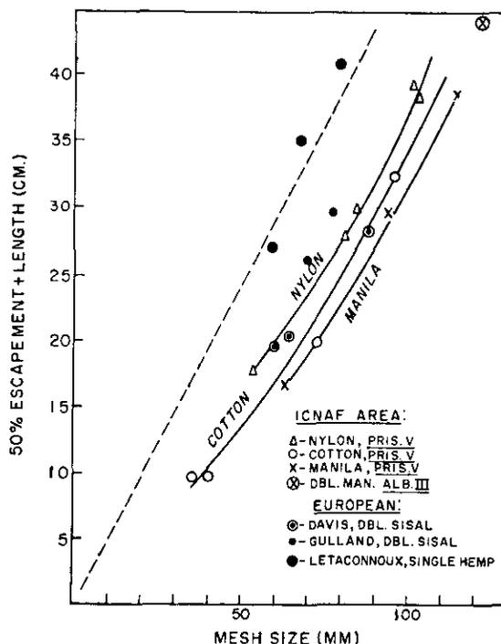
Fig. 11. Silver hake 50% retention lengths and mesh size. The dashed line represents mesh circumference = fish girth (for *M. bilinearis*).
