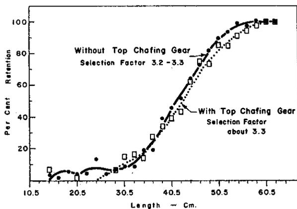
Fig. 2. Selection curves for 5-inch mesh, double-strand, manila codend with and without top chafing gear.
