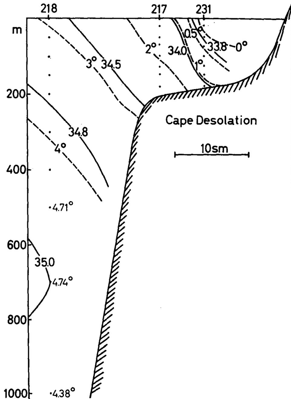
Fig. 5. Hydrographic section off Cape Desolation, 2-8 March 1962. Salinity ‰ - solid lines; temperature °C - broken lines.
