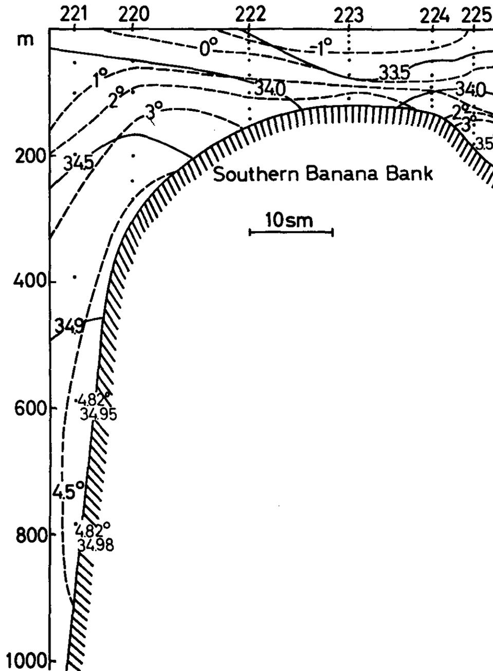
Fig. 4. Hydrographic section across southern Banana Bank, 4-5 March 1962. Salinity ‰ - solid lines; temperature  $^{\circ}\text{C}$  - broken lines.
