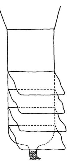
Fig. 1. Diagram showing attachment of flap-type chafers to cod-end.
