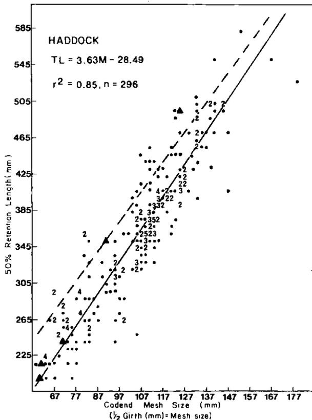
Fig. 4. General selection pattern for haddock based on historical mesh selection studies. (Each dot represents a single observation and numbers indicate points with two or more observations; triangles indicate points from the 1977 studies; the dashed line represents the length-girth relationship. The scatter graphs used throughout this paper are computer plots and as such have lower resolution than was found in the original data.)
