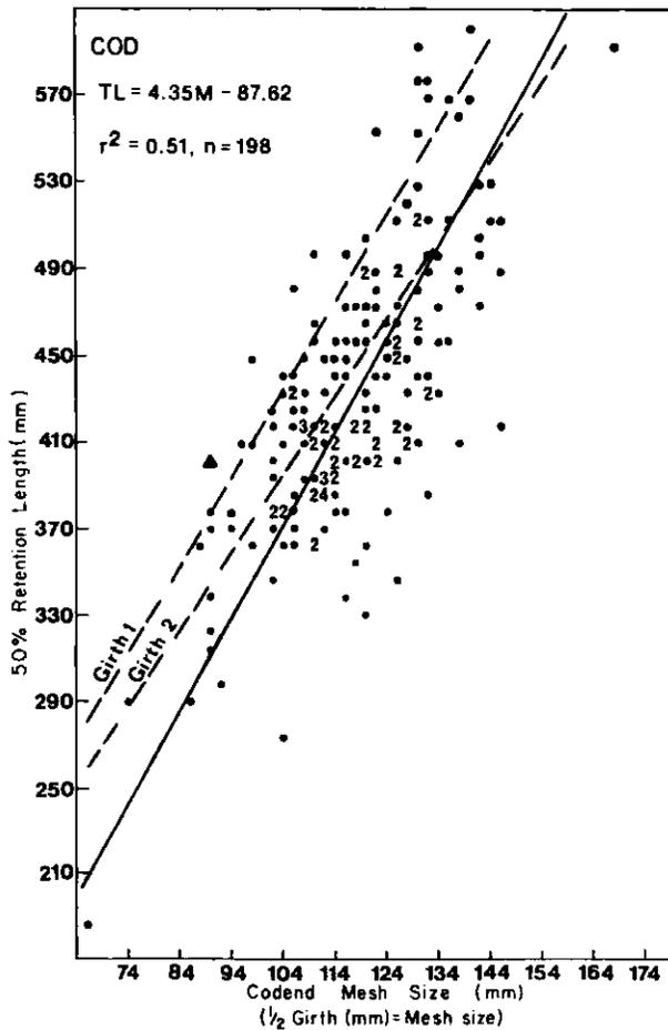
Fig. 6. General selection pattern for cod based on historical mesh selection studies. (Girths 1 and 2 are described in the text; other descriptors are the same as for Fig. 4.)
