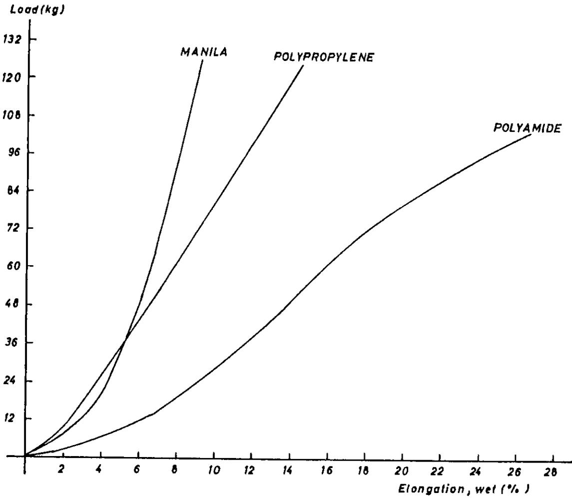
Fig.1 : Load- elongation curves for the twines used
