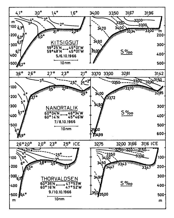
Fig. 1. Hydrographic sections off South Greenland (temperature and salinity) in October 1966.
