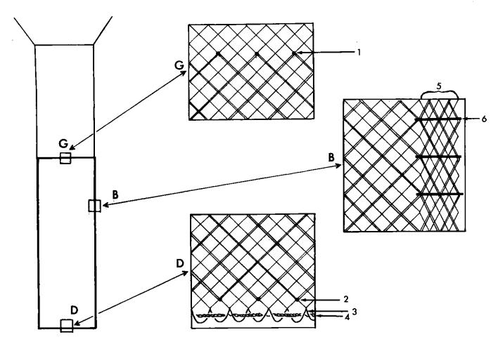
Polish-type (large-mesh) chafer showing method of rigging
