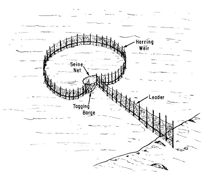
Fig. 1. Typical herring weir in which the trapped herring have been seined prepatory to pumping into a commercial carrier. The tagging barge is positioned in the mouth of the weir. After 2500-3500 fish are dip-netted into the barge, it will be towed offshore for the actual tagging.
