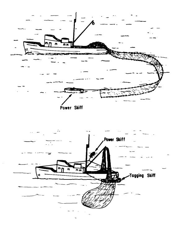
Fig. 3. Purse seine boat setting its seine in the normal manner and subsequently when the tagging operation is underway. The power skiff hauls the seiner off the partially deployed seine if necessary.
