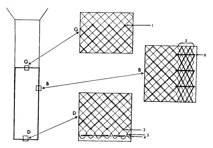
Polish-type (large-mesh) chafer showing method of rigging
