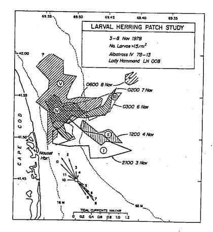
Figure 2. Delineation of the five larval herring patch mappings, 3-8 November 1978, by the vessels ALBATROSS IV and LADY HAMMOND. The patch contours represent areas where densities of larvae were greater than 15/m<sup>2</sup>. Hourly directions and velocities of the tidal currents are shown by arrows. The figures at the arrow heads are the hours after the time of maximum flood at Pollock Rip Channel.
