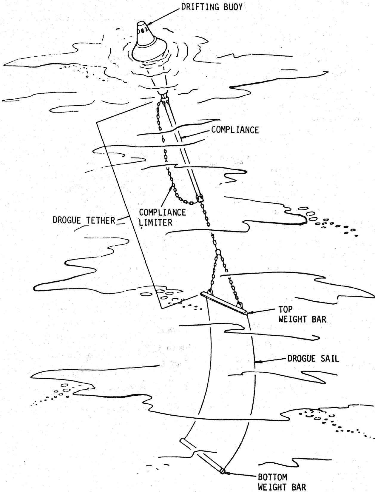
Figure 1 Schematic diagram of a drogued drifting buoy.
