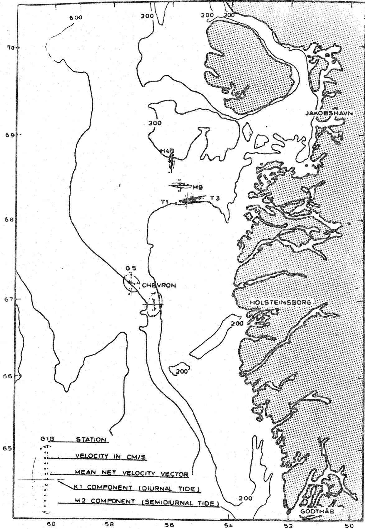
Figure 24. Tidal hodographs for  $K_1$  and  $M_2$  components for the depth interval 260-410 m.
