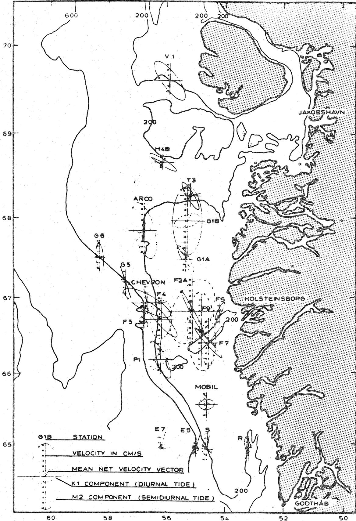
Figure 22. Tidal hodographs for  $K_1$  and  $M_2$  components for the depth interval 20-57 m.
