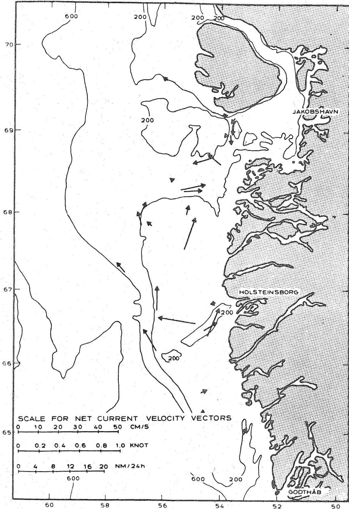
Figure 16. Net current velocity vectors for the depth interval 60-240 m.
