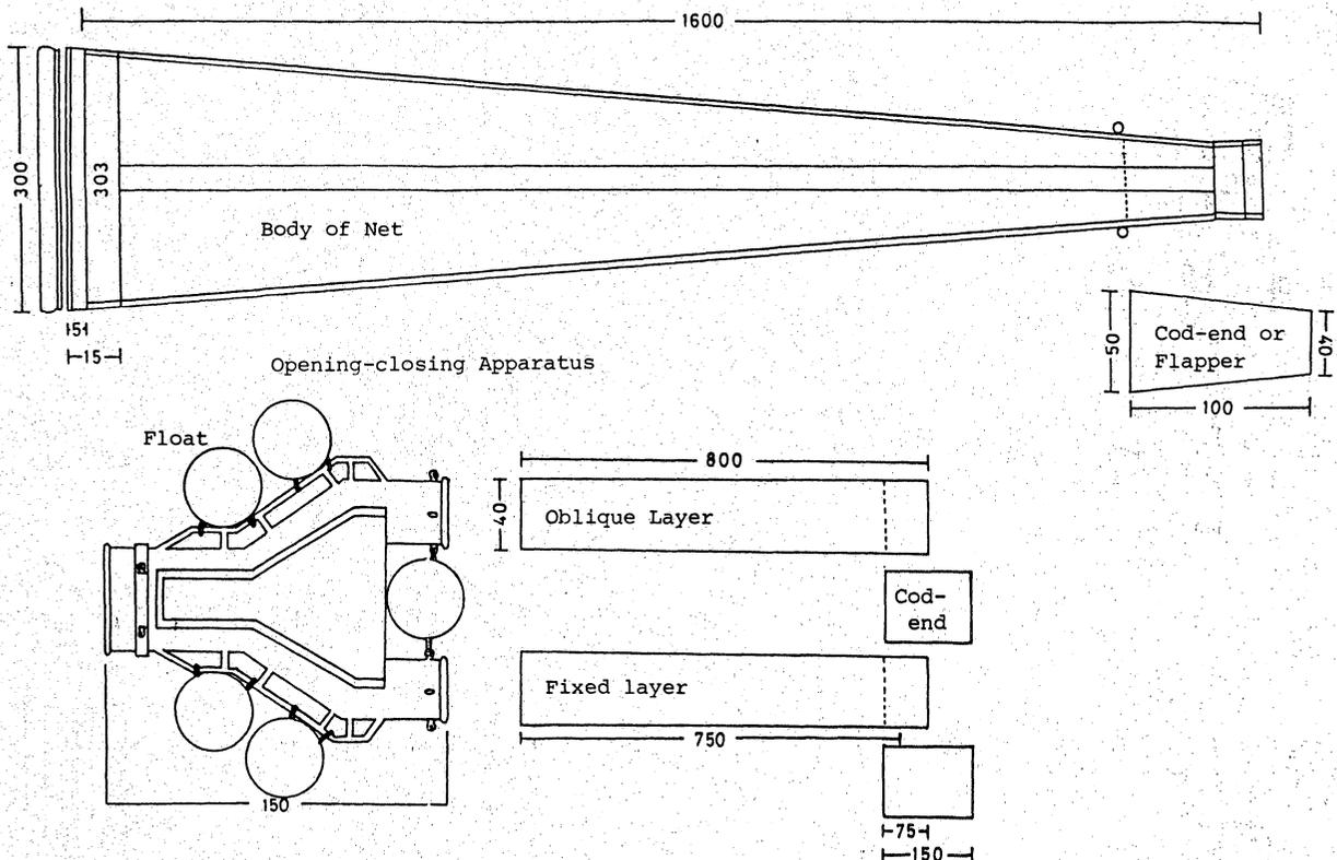
Appendix Fig. 2. KYMT type rectangular net and the opening-closing apparatus. The latter is used for depth-stratified sampling. Numerals in the figure show the length in cm.
