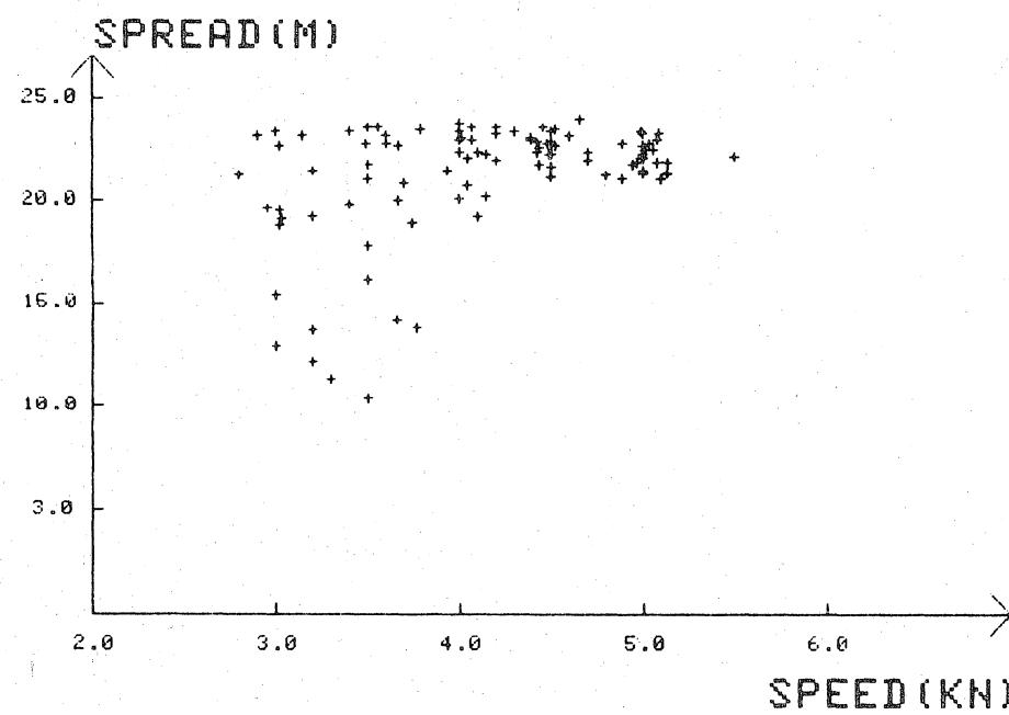
Fig. 4a,4b: 140°BT, headline height and wing spread
