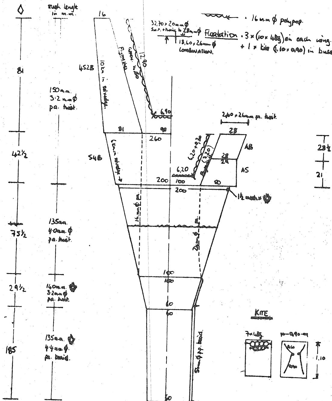
Fig. 1: 140'BT Netting and Frame Lines
