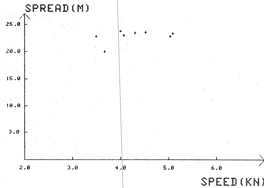
Fig. 5a,5b: 140'BT, headline height and wing spread
