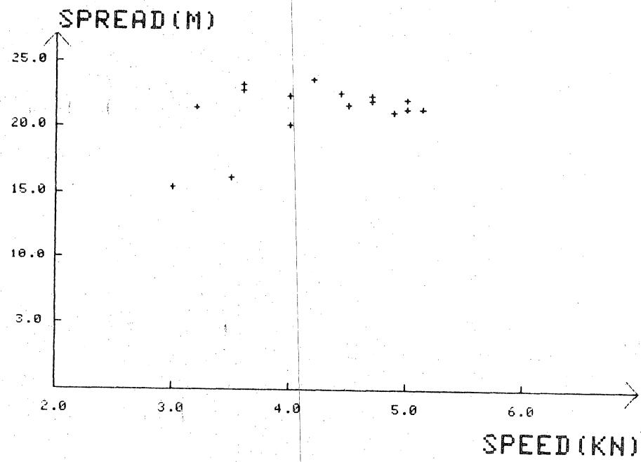
Fig. 9a,9b: 140' BT, headline height and wing spread
