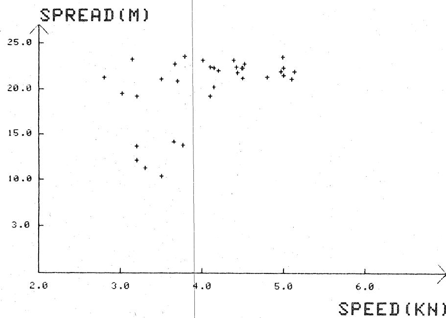
Fig. 7a, 7b: 140' BT, headline height and wing spread
