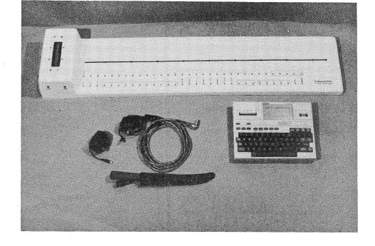
Figure 3. Photograph of digital fish measuring board developed du:
