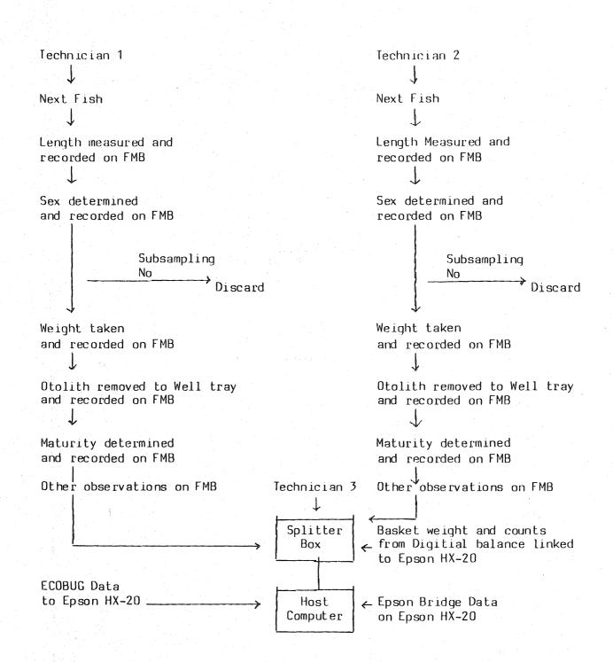
Figure 5. Sequence of events used during detailed fish sampling with electronic data acquisition system.
