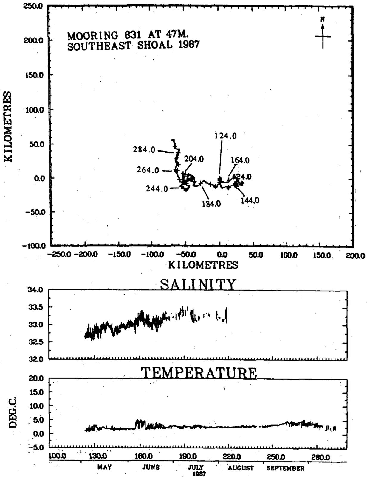
Figure 9. Progressive vector diagram and time series plots of salinity and temperature from raw data at the 47-m level at the western site (mooring 831) in 1987. Days are marked at 20-dy intervals on the progressive vector diagram.
