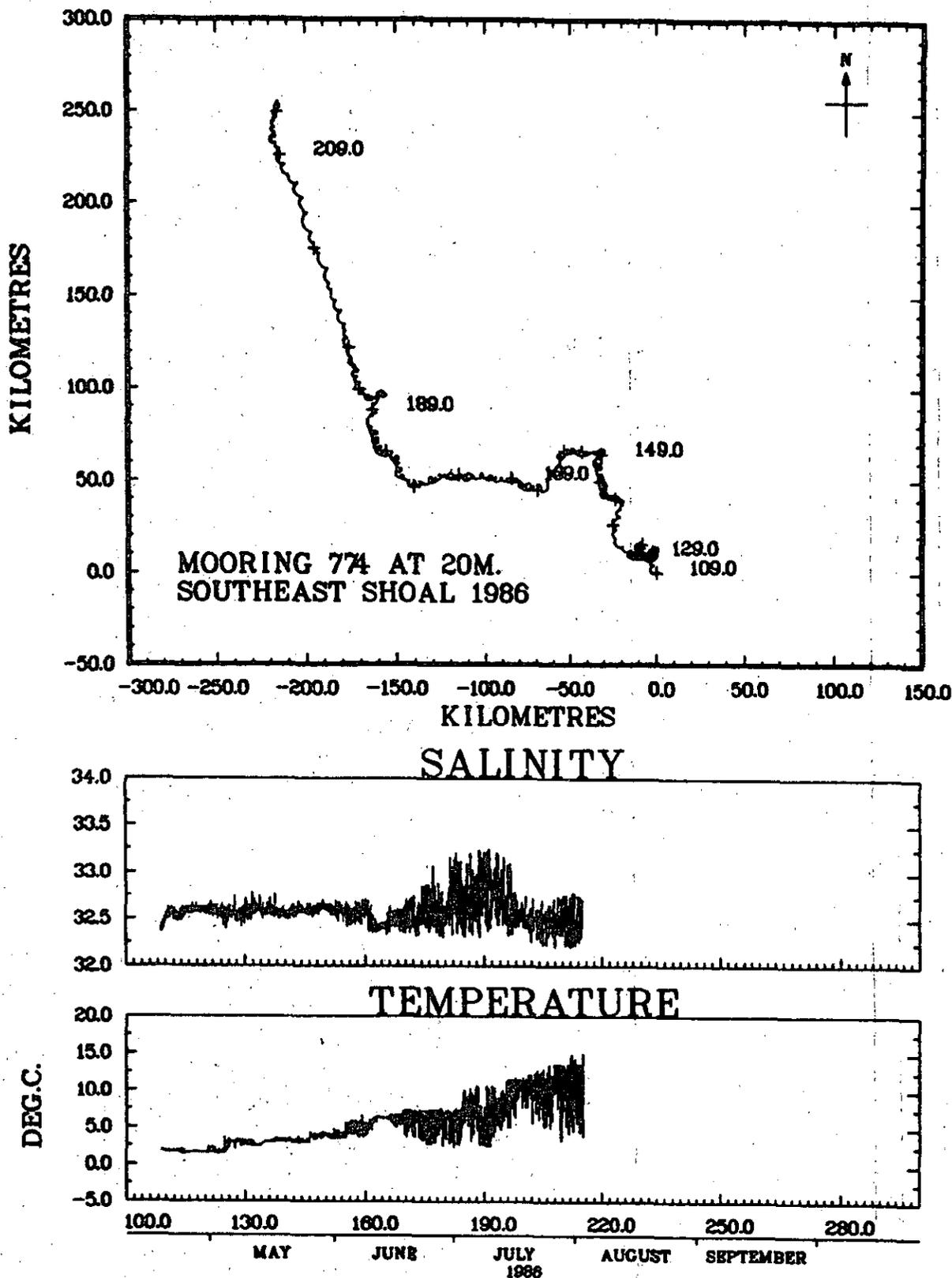
Figure 4. Progressive vector diagram and time series plots of salinity and temperature from raw data at the 20-m level at the central site (mooring 774) in 1986. Days are marked at 20-dy intervals on the progressive vector diagram.
