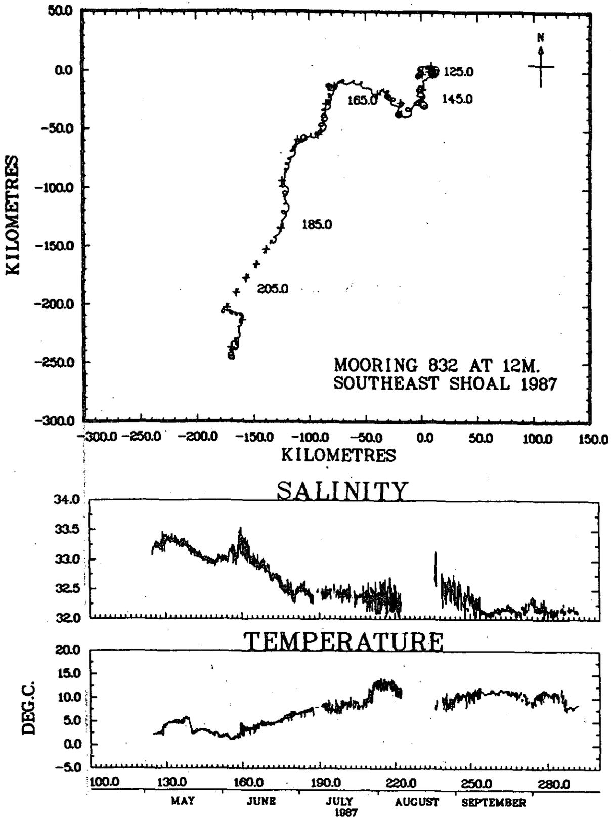
Figure 10. Progressive vector diagram and time series plots of salinity and temperature from raw data at the 12-m level at the eastern site (mooring 832) in 1987. Days are marked at 20-dy intervals on the progressive vector diagram. There is a gap in the current record during which the record-mean values are used.
