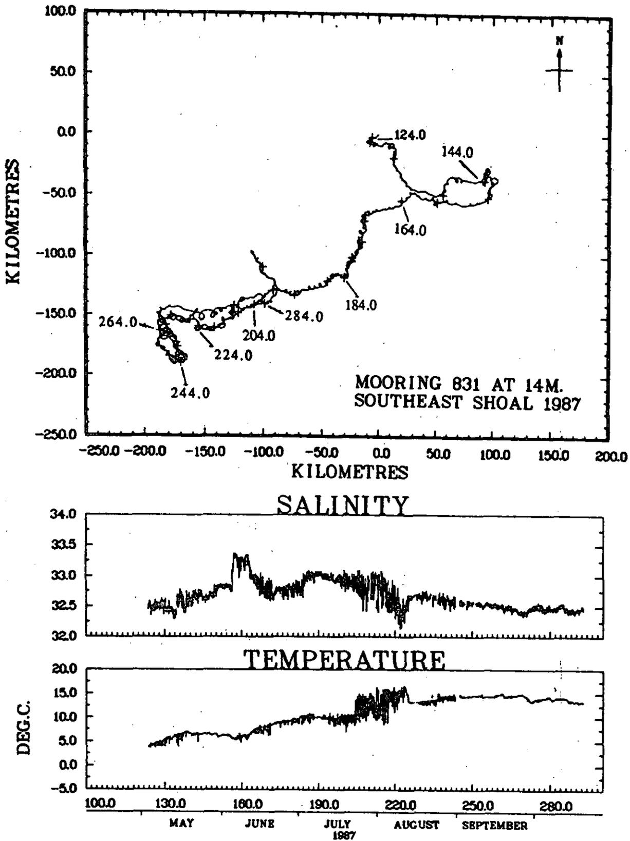
Figure 8. Progressive vector diagram and time series plots of salinity and temperature from raw data at the 14-m level at the western site (mooring 831) in 1987. Days are marked at 20-dy intervals on the progressive vector diagram.
