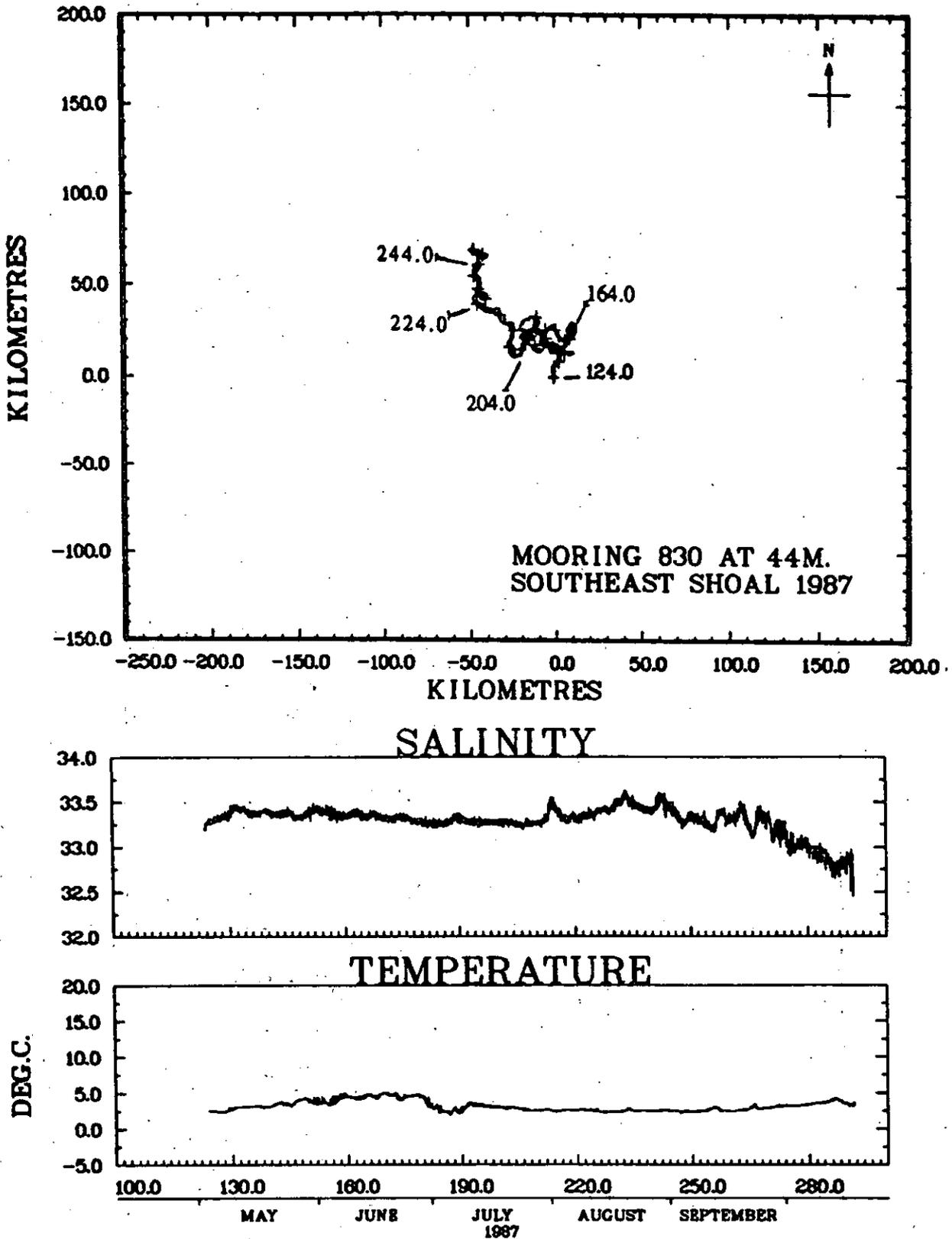
Figure 7. Progressive vector diagram and time series plots of salinity and temperature from raw data at the 44-m level at the central site (mooring 830) in 1987. Days are marked at 20-dy intervals on the progressive vector diagram.
