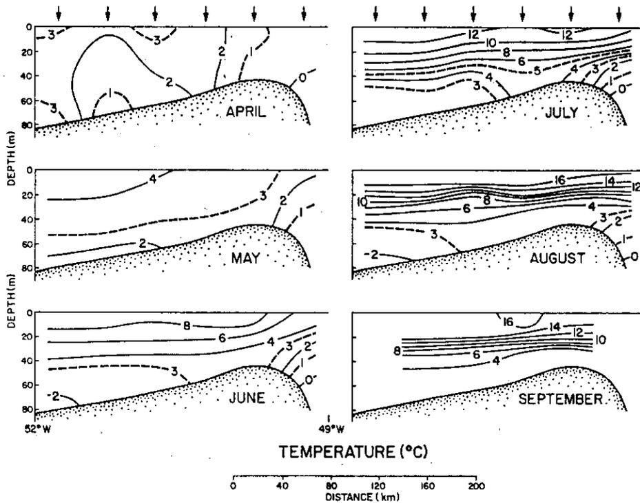
Figure 2. Seasonal evolution of the climatological temperature distribution on a vertical west-east section across Southeast Shoal. Contours are based on the MEDS long-term monthly-means for 1/2 x 1/2 degree areas between 44°N and 44°30'N.
