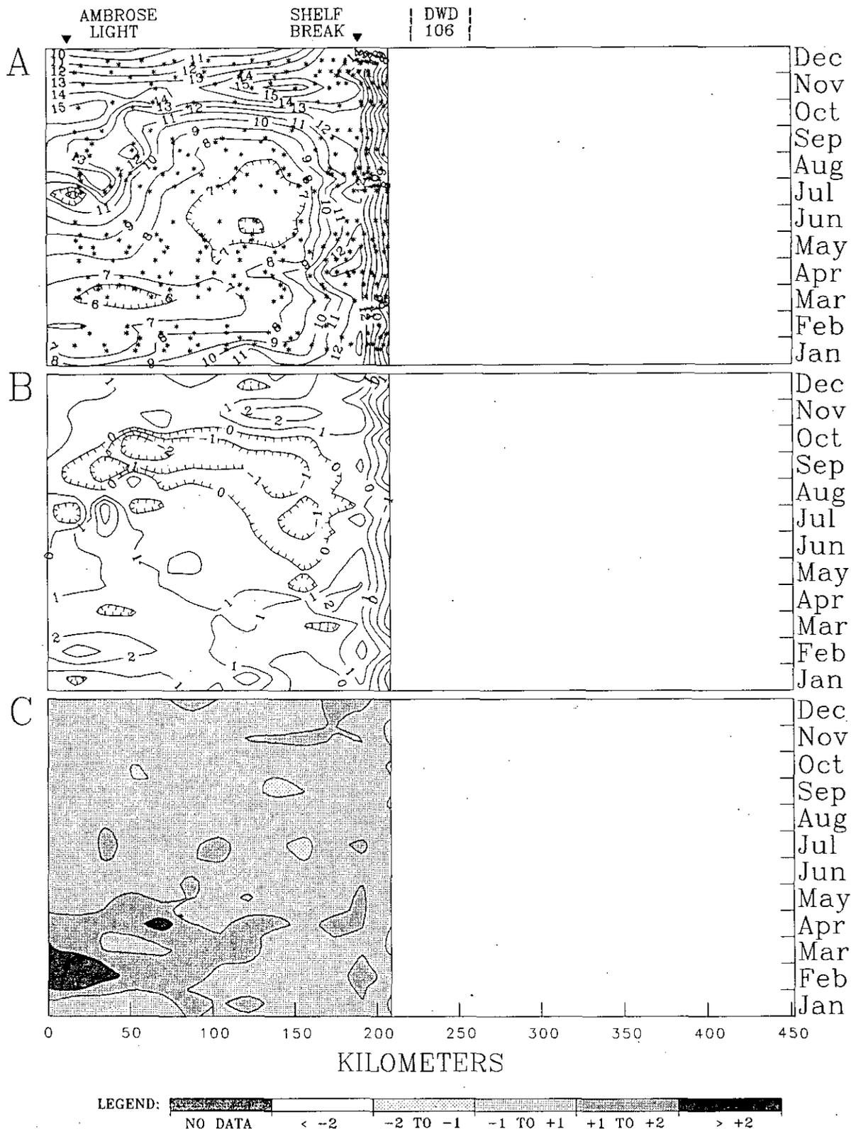
Figure 4. Bottom temperature conditions along the Middle Atlantic Bight transect during 1991. A. Measured values (degrees centigrade) in time and space. Dots indicate sampling locations. B. Anomalies in time and space based on 1978 through 1991 means. C. Standardized anomalies (standard deviations) in time and space based on 1978 through 1991 means and variances. In panels A and B values decline on those sides of contour lines with hachures.
