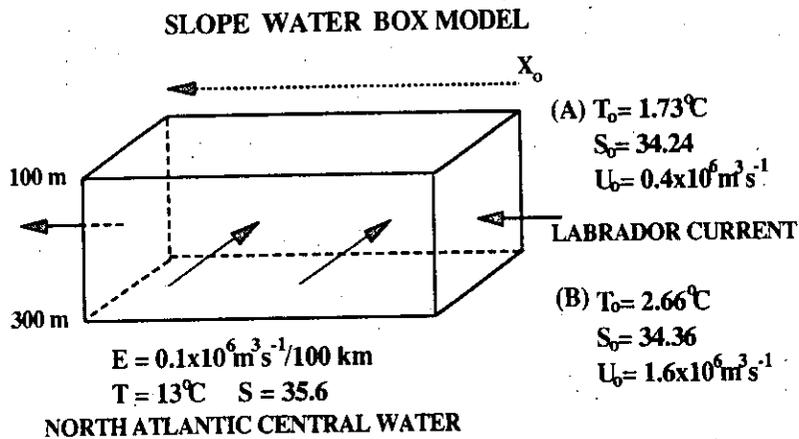
Fig. 11. Box model of slope water where X is located at Section A4 (Fig. 1). The Labrador Current water properties and transport are given as (A) and (B) and correspond to a warm and cold year respectively, on the Scotian Shelf. The entrainment rate, E, temperature and salinity of North Atlantic Central Water are taken as constant.
