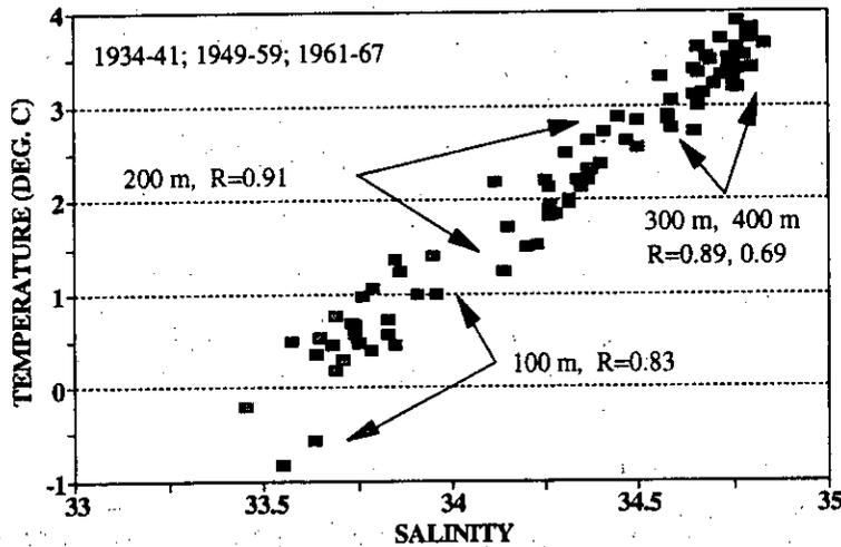
Fig. 9. Average temperature and salinity of the Labrador Current Water at 4 depths (100, 200, 300 and 400 m) from the period 1934-67. The years that data were collected and the T-S correlations (R) are shown.
