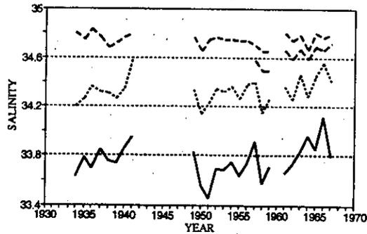
Fig. 8. Average temperature and salinity of the Labrador Current waters at 100, 200, 300 and 400 m from U.S. Coast Guard surveys (see Morgan, 1969, for example).
