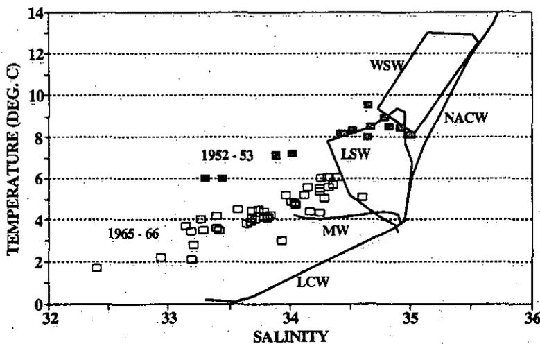
Fig. 3. Temperature-salinity diagram of observations from depths  $\geq 100$  m for a warm (1952-53, solid box) and cold (1965-66, open box) period. The envelopes of T-S characteristics for Warm Slope Water (WSW) and Labrador Slope Water (LSW) (from Gattien, 1976), and the average curves (Morgan, 1969) for North Atlantic Central (NACW), Mixed (MW) and Labrador Current Water (LCW) are also shown.
