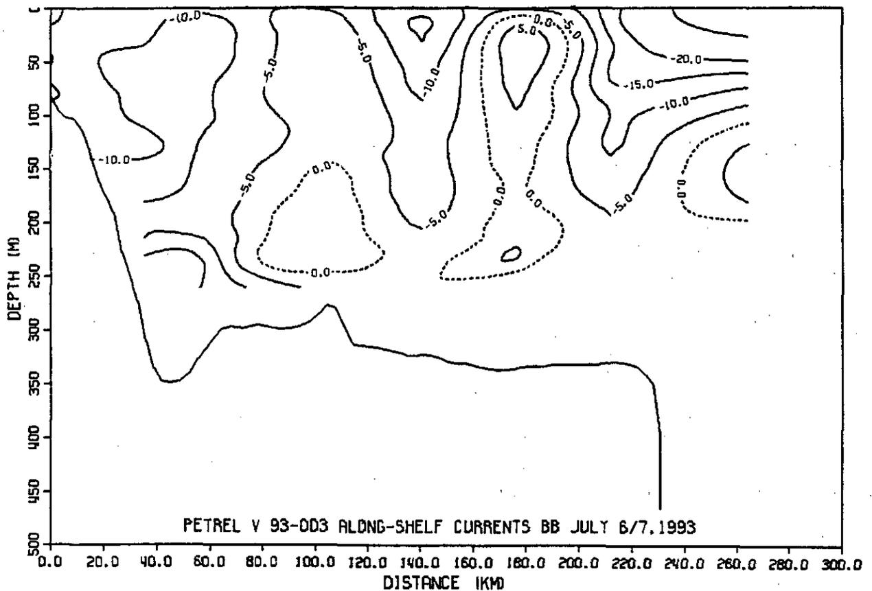
Fig. 13. The vertical distribution of the current field along the Cape Bonavista transect. Negative currents are southward, from an ADCP survey.
