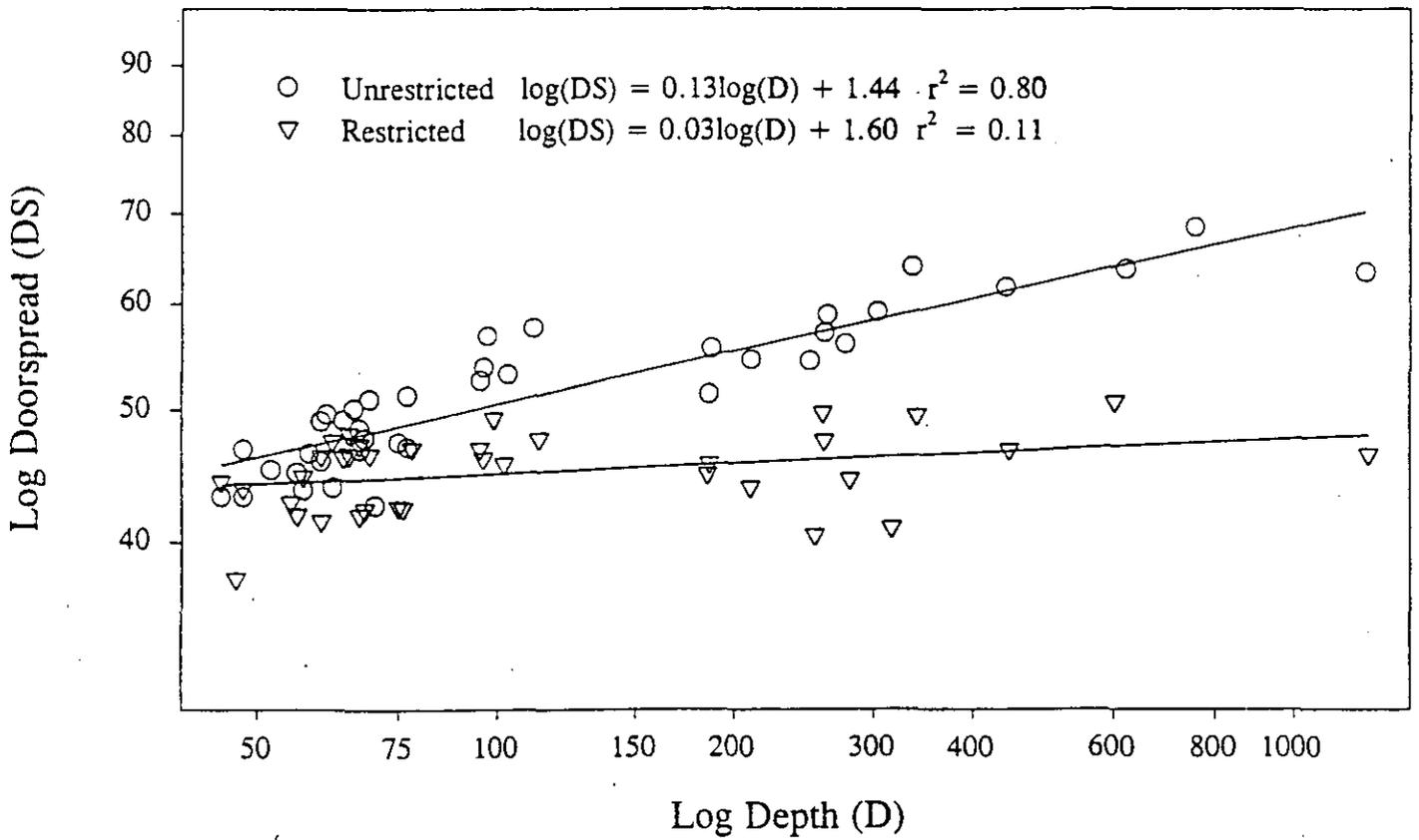
Fig. 4 Relationship of unrestricted and restricted door spread with depth.
