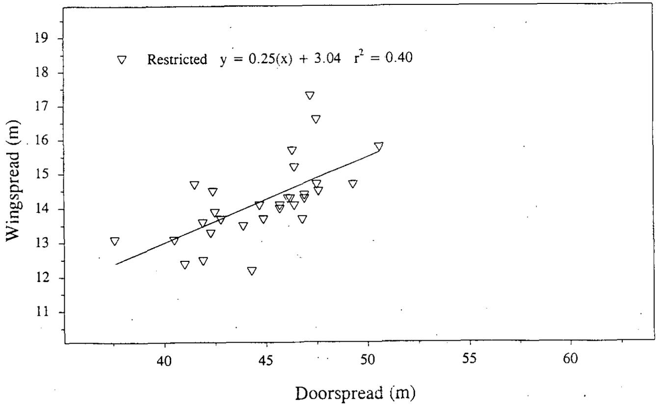
Fig. 6 Relationship between wing spread and door spread for unrestricted and restricted trawl hauls.
