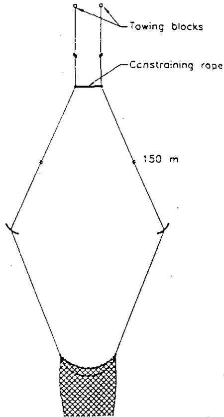
Fig. 3 Rigging diagram and technique used to restrain door spread (reprinted from Engas and Ona 1991).
