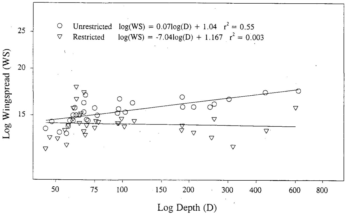
Fig. 5 Relationship of unrestricted and restricted wing spread with depth.
