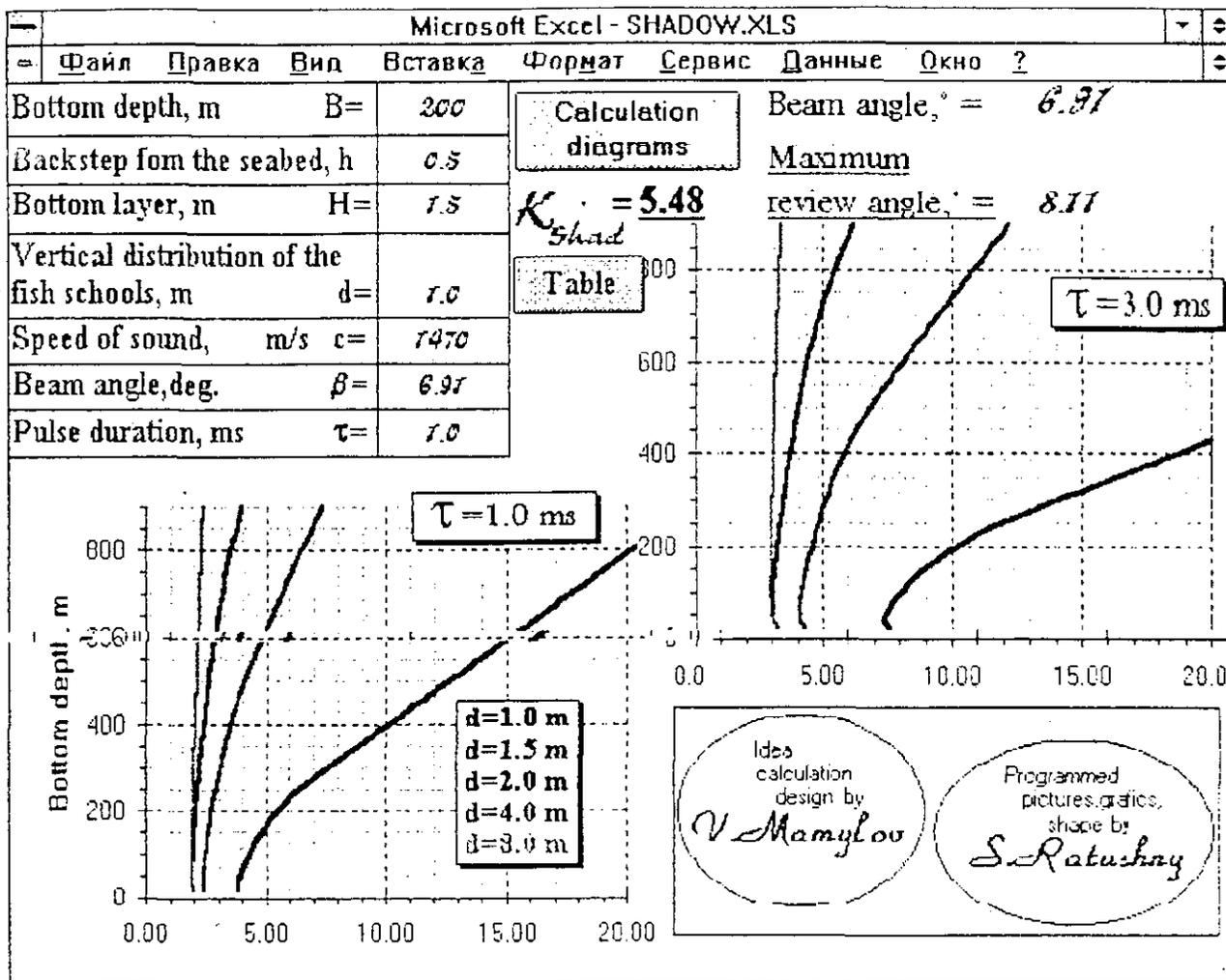
Figure 8. The MicroSoft Excel window with the activated program of estimation of the shadow zone coefficients
