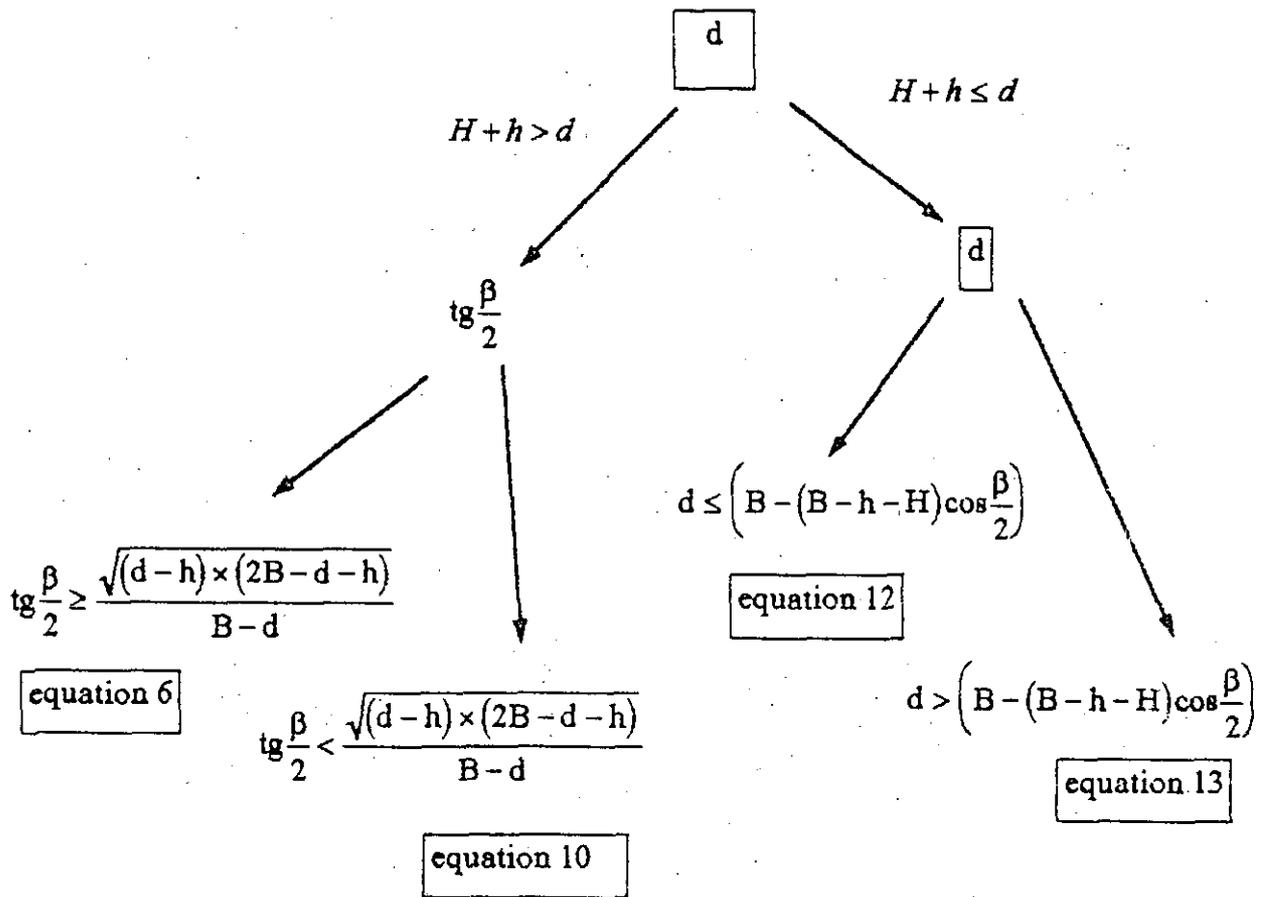
Figure 5. Algorithm of choice of a method of estimation  $K_{shad}$
