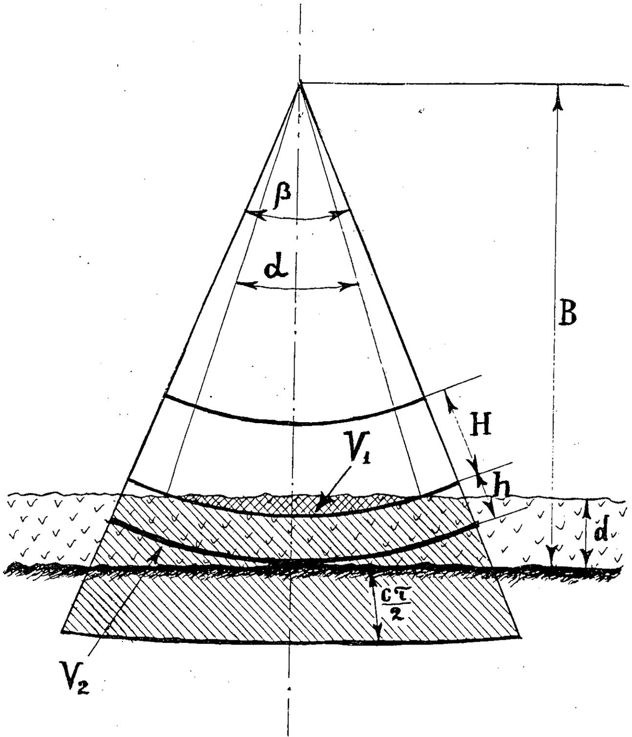
Figure 1. Algorithm of estimation  $K_{\text{shad}}$  at  $H+h>d$  and  $\alpha<\beta$
