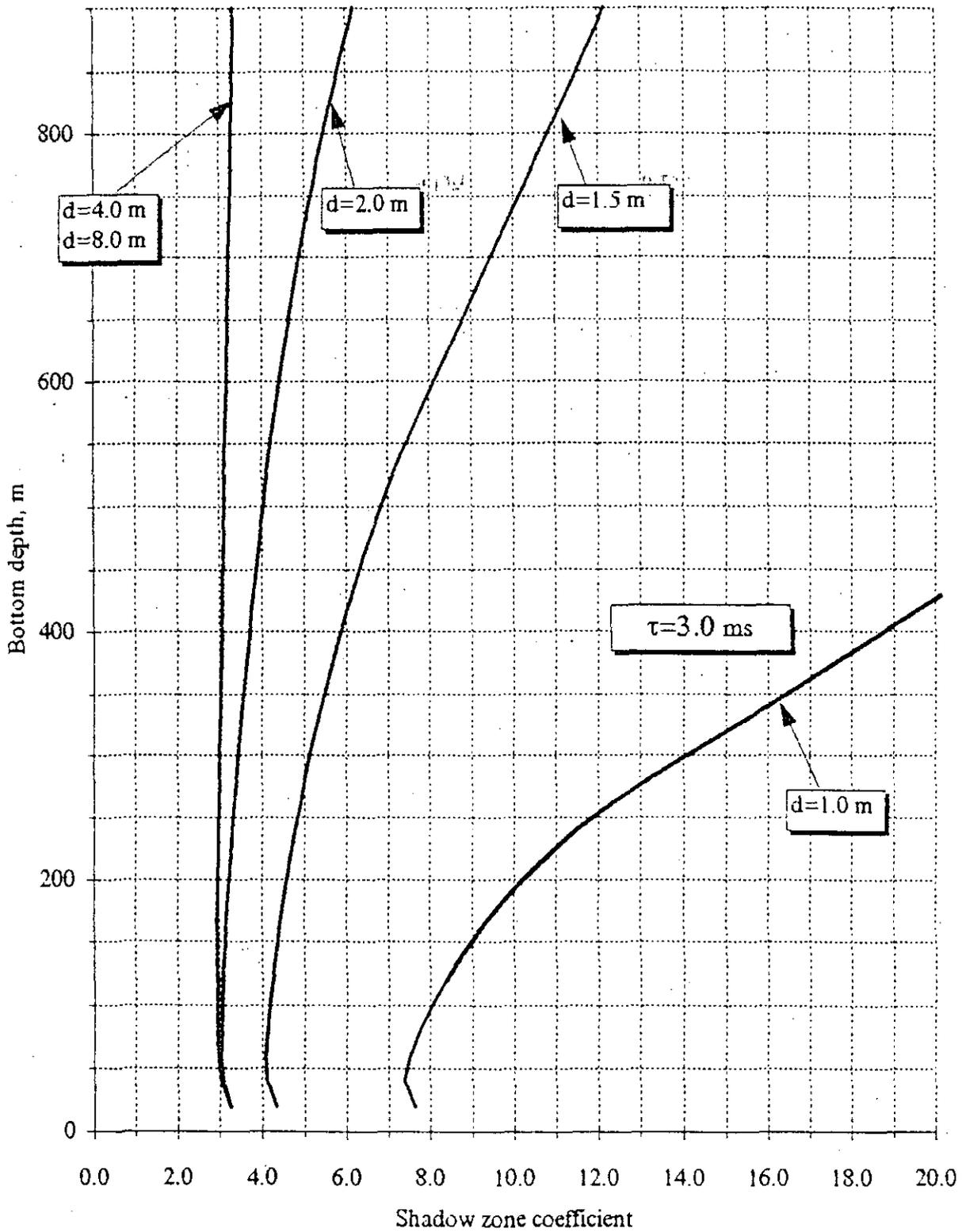
Figure 7. Dependences of the shadow zone coefficients for  $\tau=3,0$  ms
