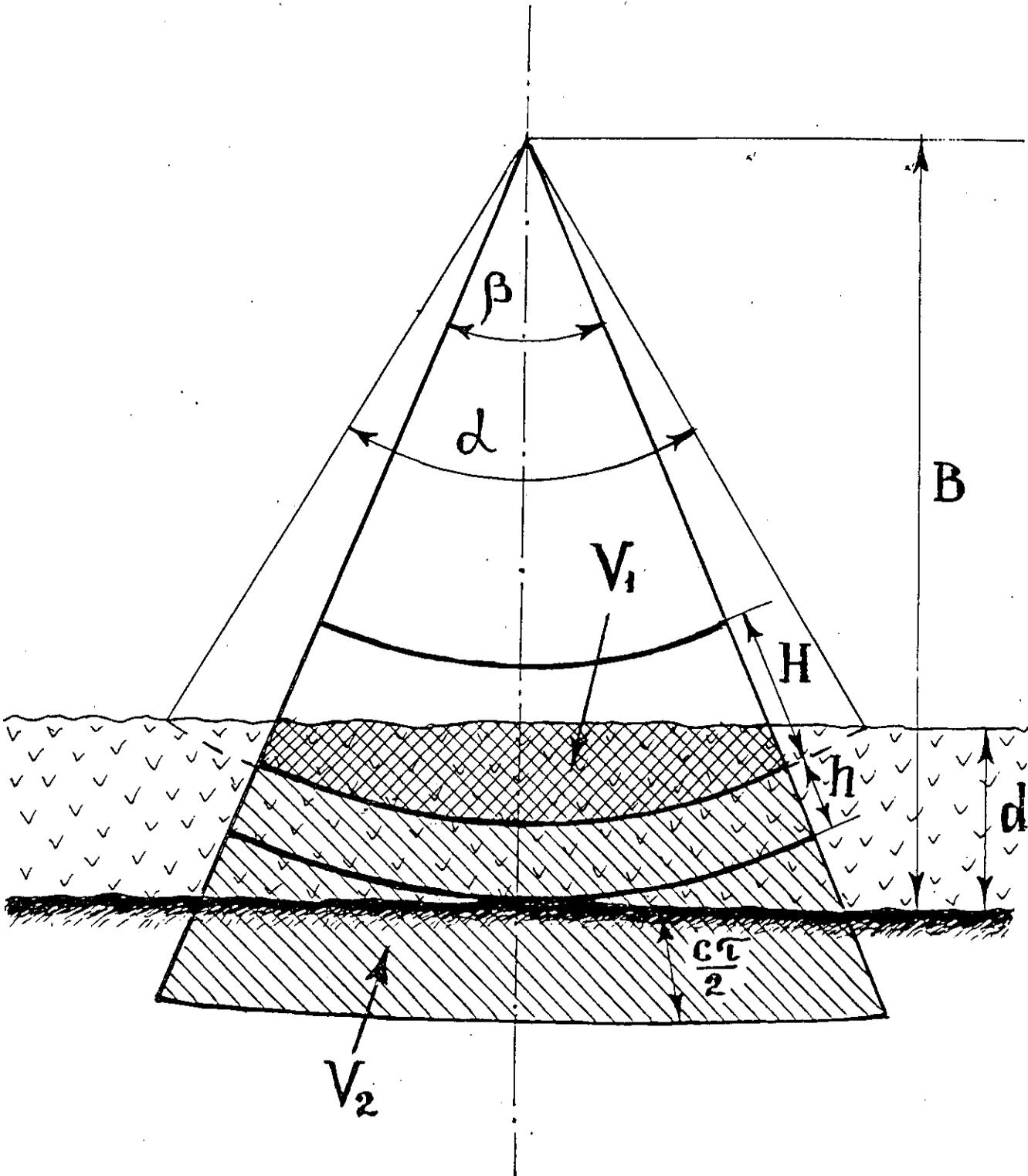
Figure 2. Algorithm of estimation  $K_{chad}$  at  $H+h>d$  and  $\alpha>\beta$
