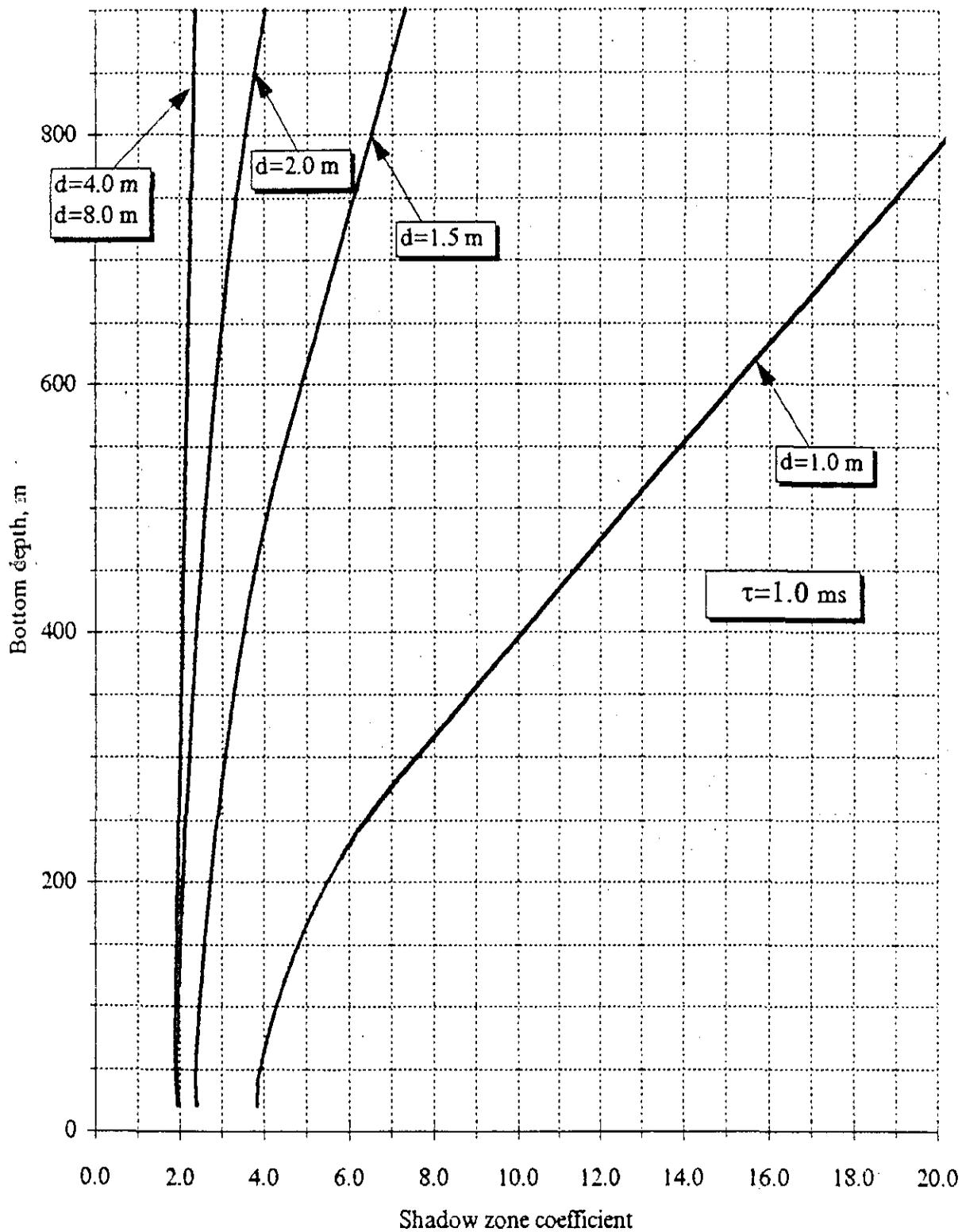
Figure 6. Dependences of the shadow zone coefficients for  $\tau = 1,0 \text{ ms}$
