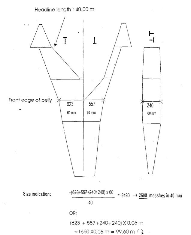
Fig. 1 The measurements of a shrimp trawl. the position where measurement should take place is indicated by "X front edge of belly". Calculations are shown on the left side.
