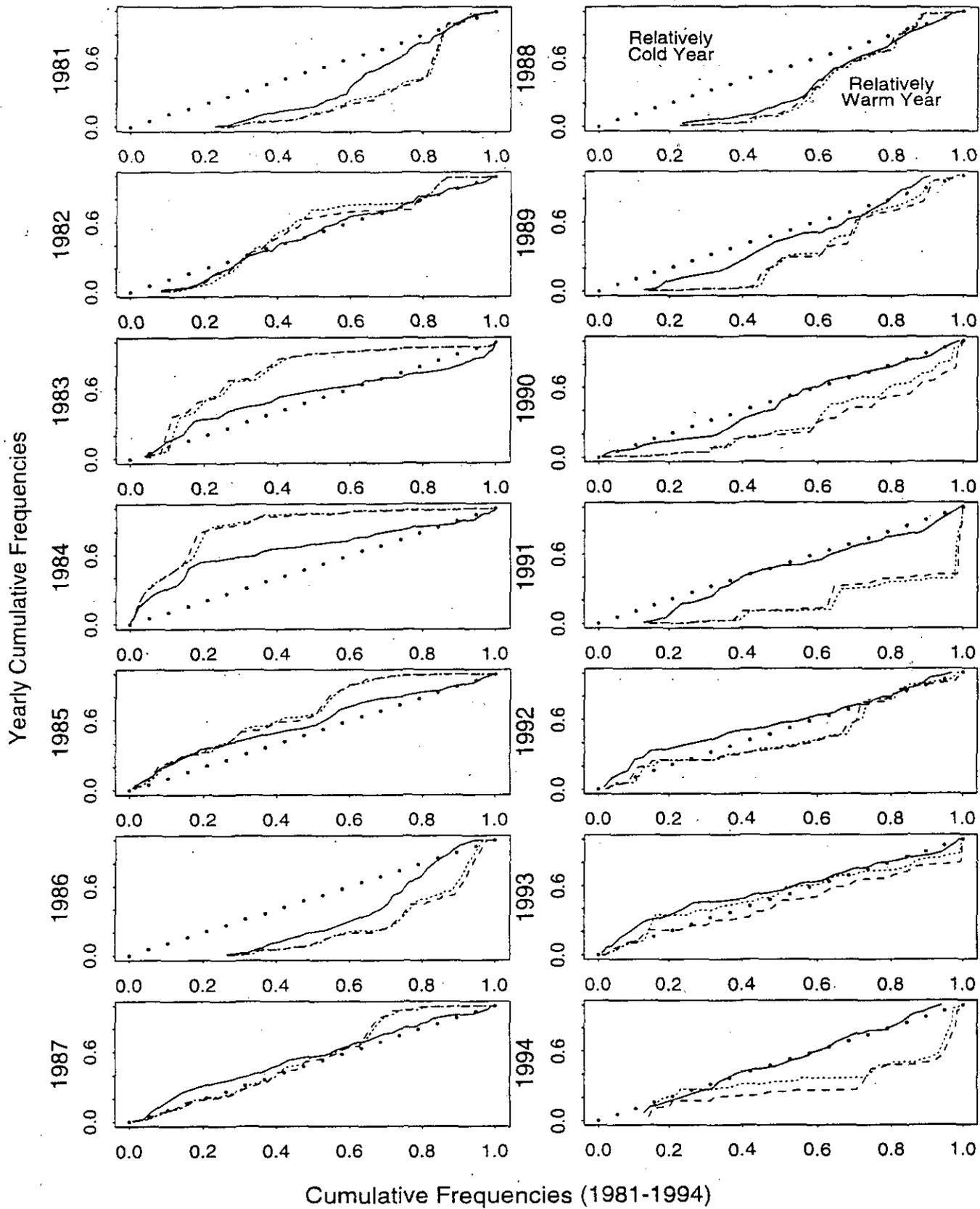
Figure 3b. Yearly weighted and unweighted bottom temperature cumulative frequency distributions versus the corresponding 1981-1994 combined distributions for the 2J trawl fall survey. The points denote a 1:1 relationship.
