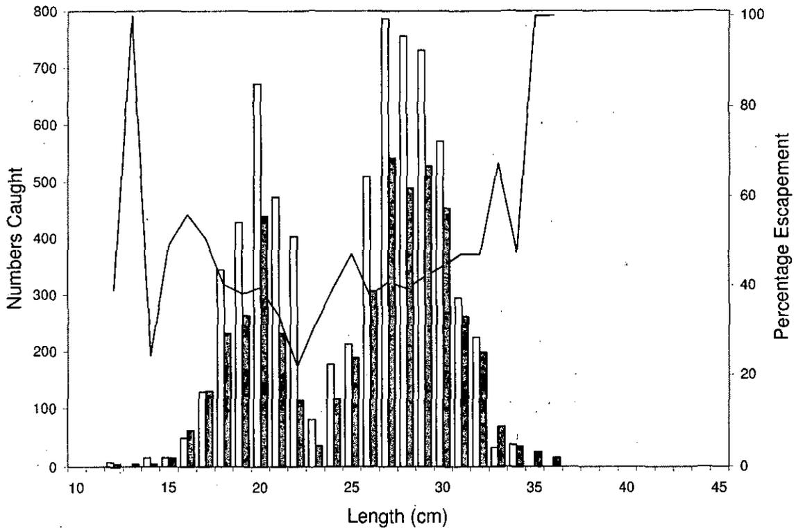
Fig. 8. *Alfred Needler* (40mm vertical grate inserted at 25 degrees): length compositions of silver hake catches in top (black bars) and bottom (white bars) codends, and estimated escapement at length (line).
