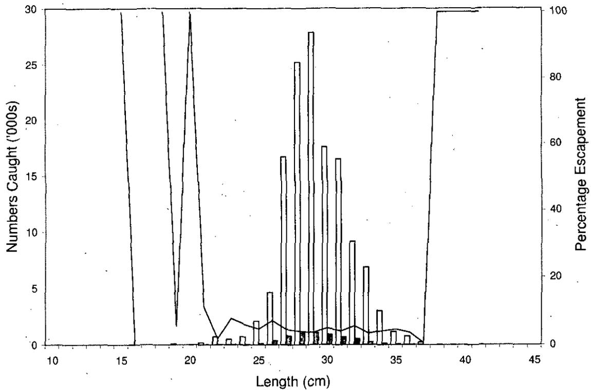
Fig. 4. *Rio Moa* (40mm vertical grate): length compositions of silver hake catches in top (black bars) and bottom (white bars) codends, and estimated escapement at length (line).
