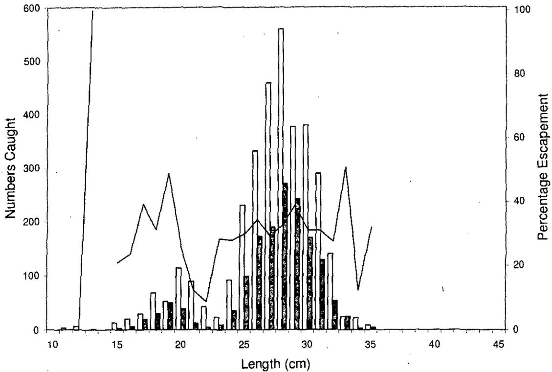
Fig. 9. *Alfred Needler* (40mm vertical grate inserted at 25 degrees and funnel 42.5cm ahead): length compositions of silver hake catches in top (black bars) and bottom (white bars) codends, and estimated escapement at length (line).
