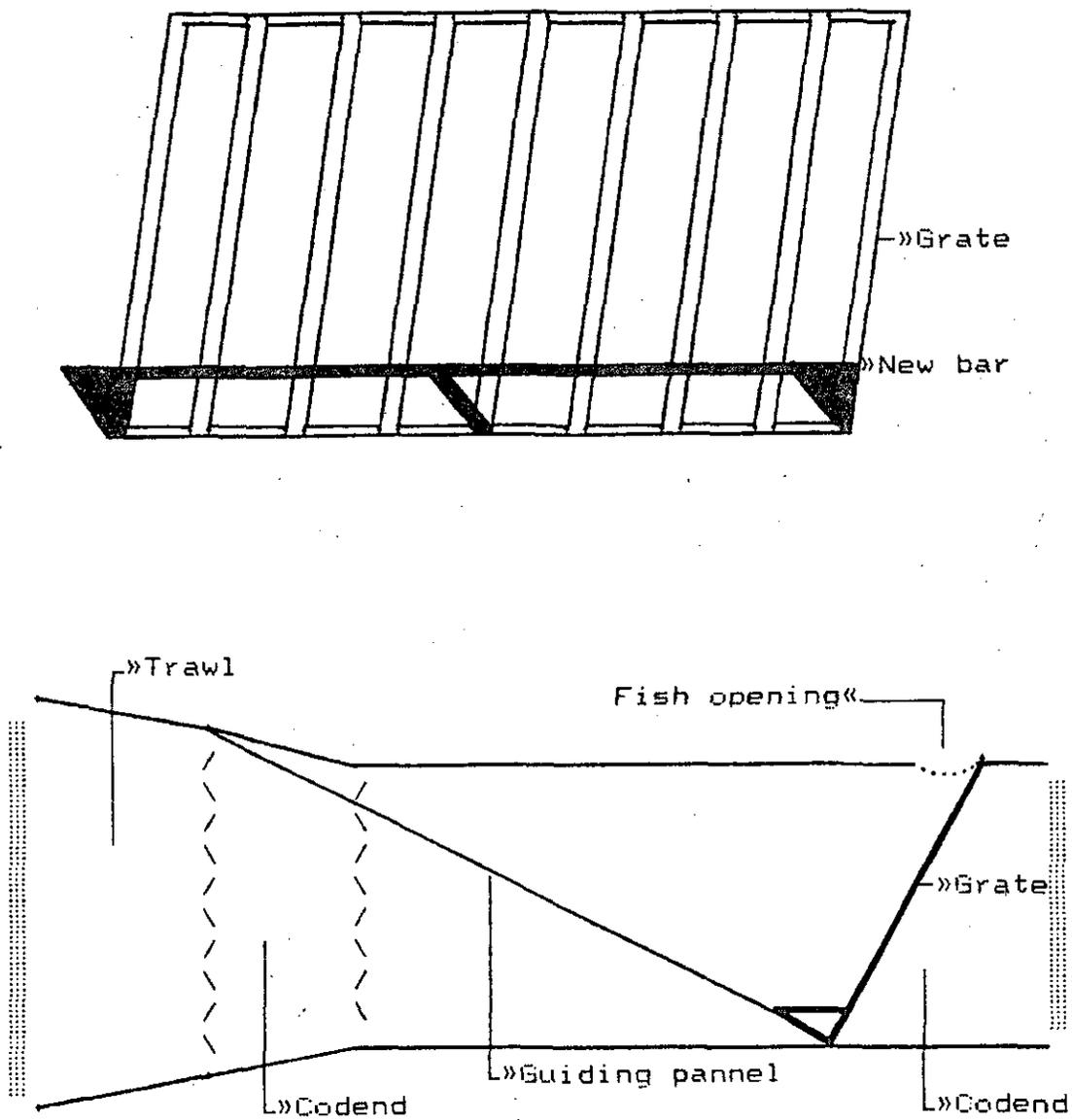
Fig. 2. Diagram illustrating the bar installed in front of the separator grate, and attachment to it of the guiding panel, used during the *Rio Moa* experiment.
