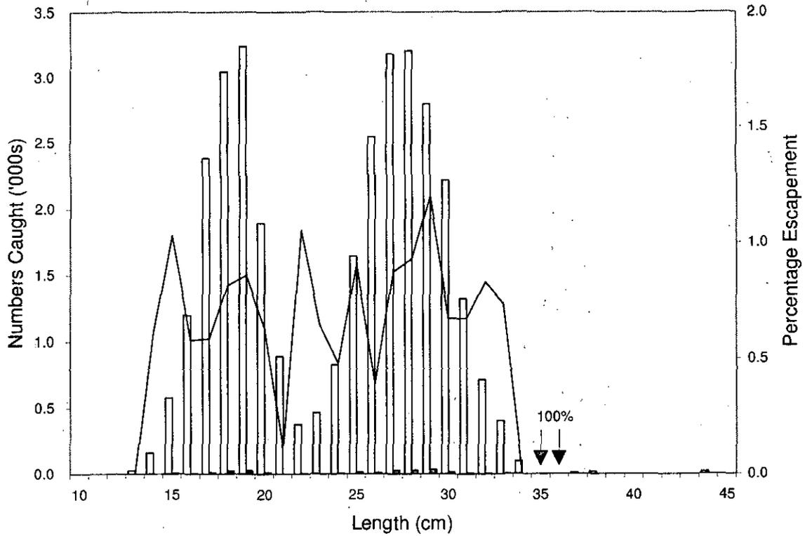
Fig. 7. *Alfred Needler* (50mm vertical grate): length compositions of silver hake catches in top (black bars) and bottom (white bars) codends, and estimated escapement at length (line). (Note percentage escapement scale.)
