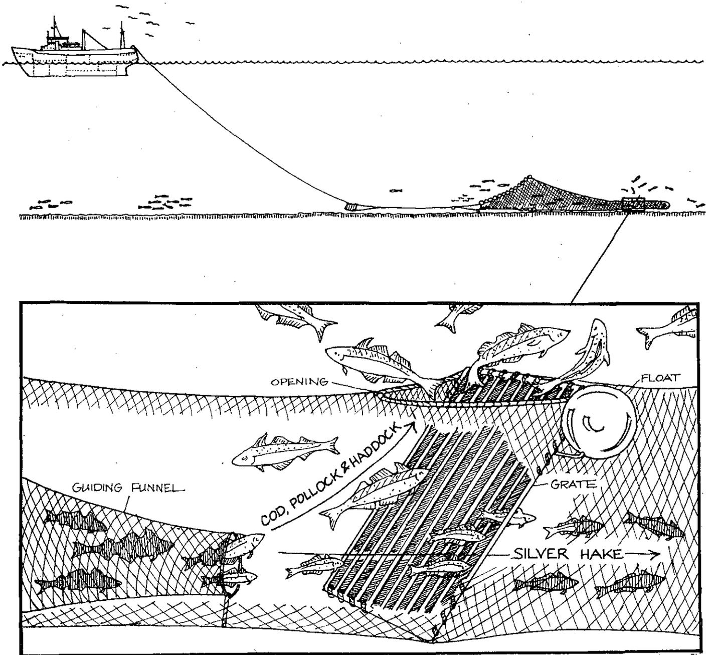
Fig. 1. Diagram illustrating the installation and operation of an otter trawl codend separator grate.
