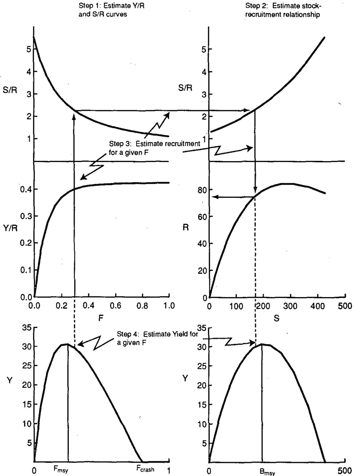
Fig. 4: Family of curves describing yield (Y) per recruit (R), spawning stock biomass (S) per recruit, and yield as a function of fishing mortality (F). The steps to relate the curves are described in the text (based on Fig. 1 of Sissenwine and Shepherd (1987)).
