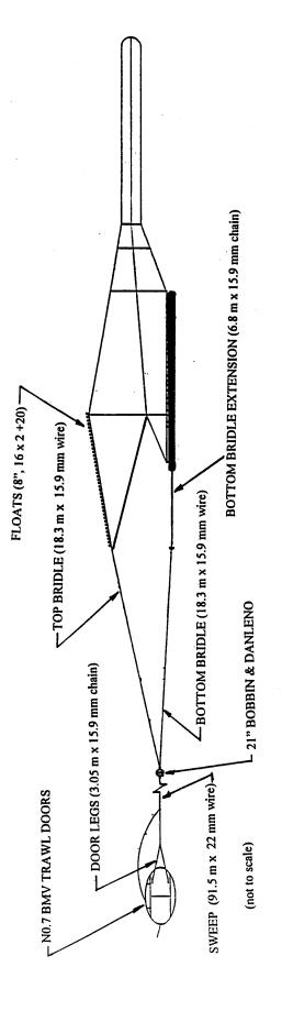
Fig. 1. Rigging diagram of the FPI Engel 145 Hi-Lift survey trawl.
