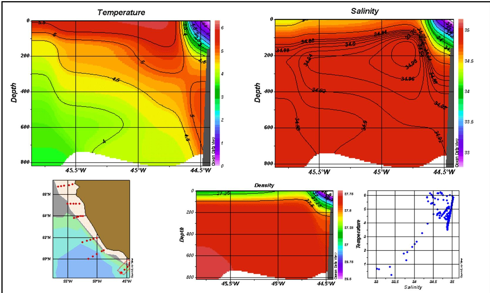
Fig. 8. Vertical distribution of temperature, salinity and density at the Cape Farewell section, 10 July 1999
