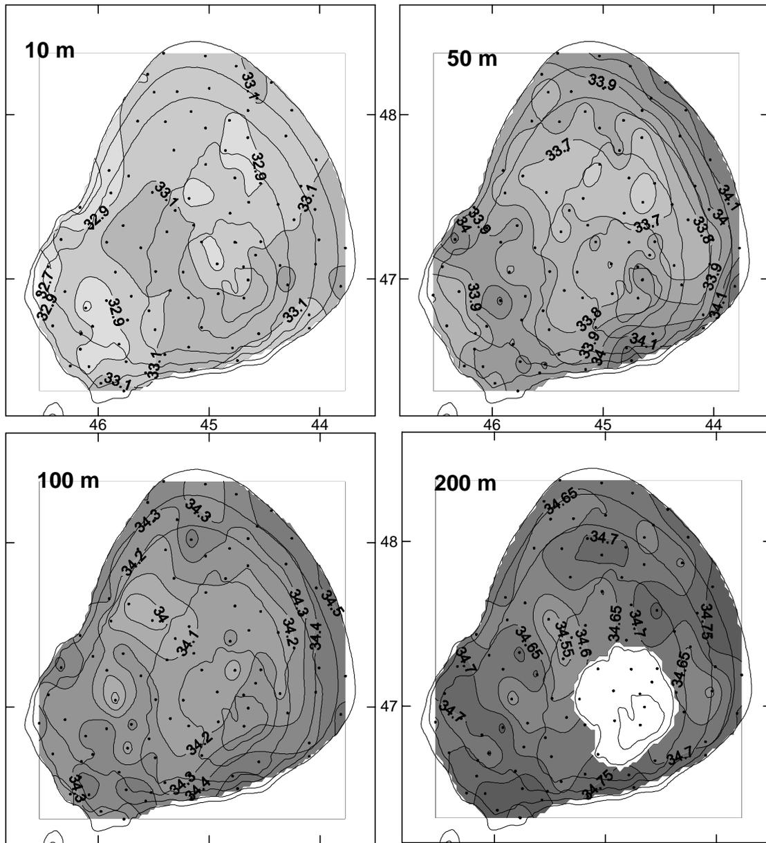
Fig. 4. Isohaline contours maps at 10, 50, 100, and 200 m depth on Flemish Cap.
