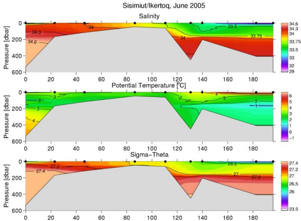
Fig. 32. Vertical distribution of temperature, salinity and density at the Ikertoq fjord, June 27-28, 2005. Sisimiut section left (identical to Fig. 19). Note, the innermost fjord station has been repeated
