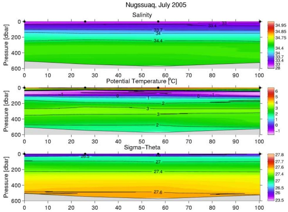
Fig. 25. Vertical distribution of temperature, salinity and density at the Nugssuaq section, July 24–25, 2005.
