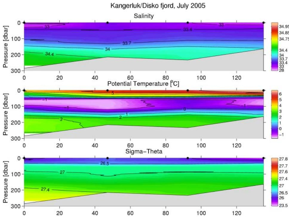
Fig. 24. Vertical distribution of temperature, salinity and density at the Kangerluk (Disko Fjord) section, July 26-27, 2005.
