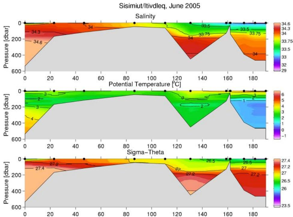
Fig. 34. Vertical distribution of temperature, salinity and density at the Itivdleq fjord, June 27-29, 2005. Sisimiut section left (identical to Fig. 19). Note, the innermost fjord station has been repeated
