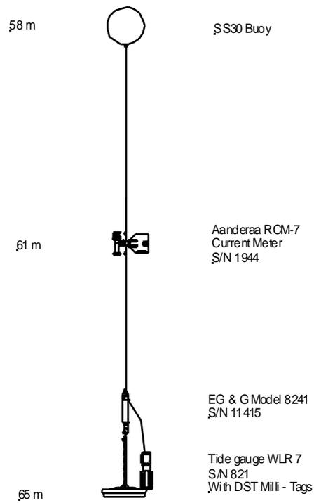
Fig. 3. Mooring layout for deployment in Division 3N showing the current meter, tidal gauge and DST tag locations relative to the bottom.
