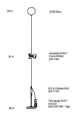
Fig. 3. Mooring layout for deployment in Division 3N showing the current meter, tidal gauge and DST tag locations relative to the bottom.
