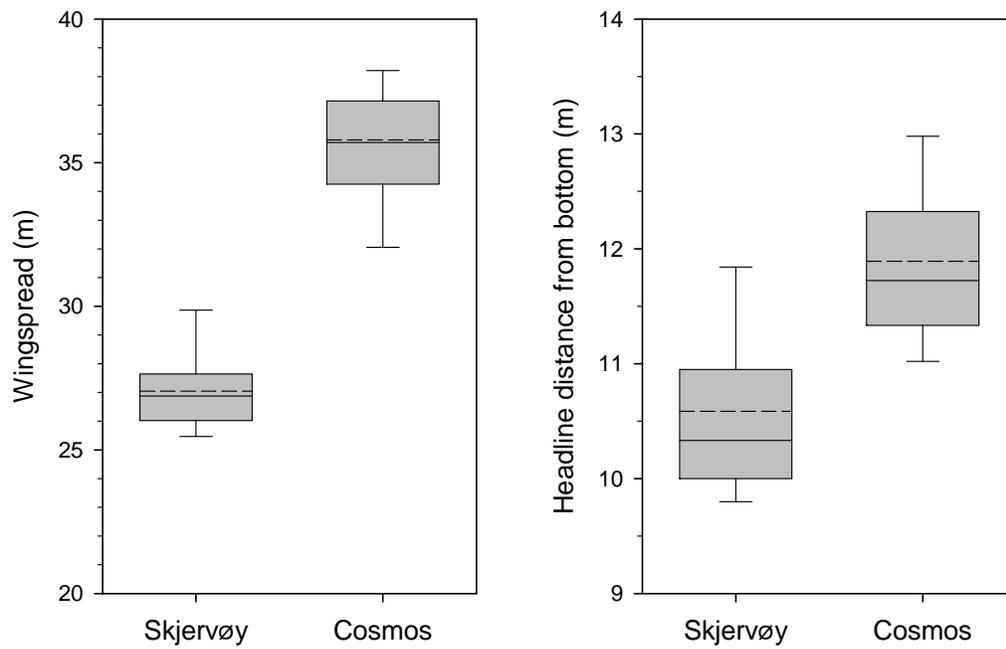
Fig. 2. Box whisker plots showing arithmetic means (stippled line) and medians (solid lines) of wingspread and headline distance to bottom for the two trawl types (*Skjervøy* 3000 and *Cosmos* 2000) with 95% confidence interval (upper and lower borders of grey box) and lower and upper quartiles (error bars) respectively. Results based on 39 hauls for each trawl (pairs of hauls made on the same track either with the *Skjervøy* or the *Cosmos* trawl first).
