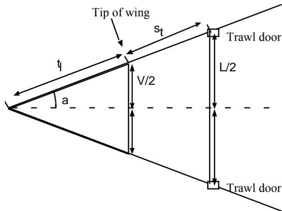
The width between trawl doors ( $L$ ) is monitored during towing by sensors ("SCANMAR HC4"). The total length of the trawl excluding the cod end ( $t_l$ ) is known (measured on land) as well as the total length between the trawl door and the tip of the wing "bridle length" ( $s_t$ ) (measured on land). Two expressions for  $\sin a$  can be formed and put equal to each other:
