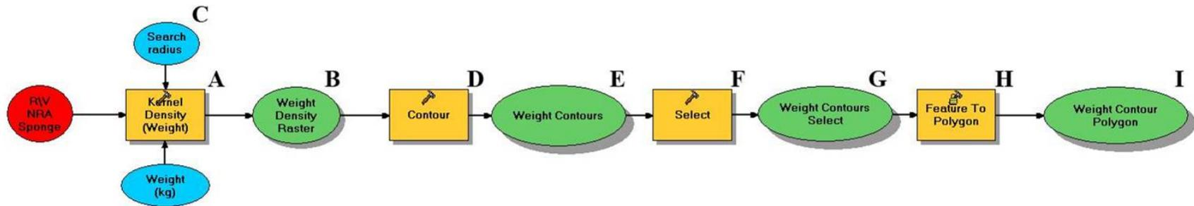
**Figure 3.** The graphic output model created in ArcGIS 9.2 used to describe sponge density in the NRA. The red circle represents the input data; orange boxes represent the ArcGIS tool utilized; blue ovals represent the adjustable variables for the tools to which they are attached; green ovals represent the output derived from each tool.
