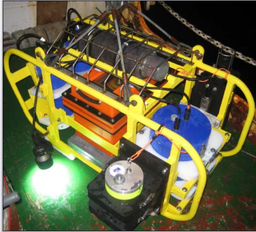
Figure 1a.13. The 4K camera system (4KCam) used to conduct the in situ benthic surveys in the Sackville Spur area was built by the Geological Survey of Canada (GSCA).
