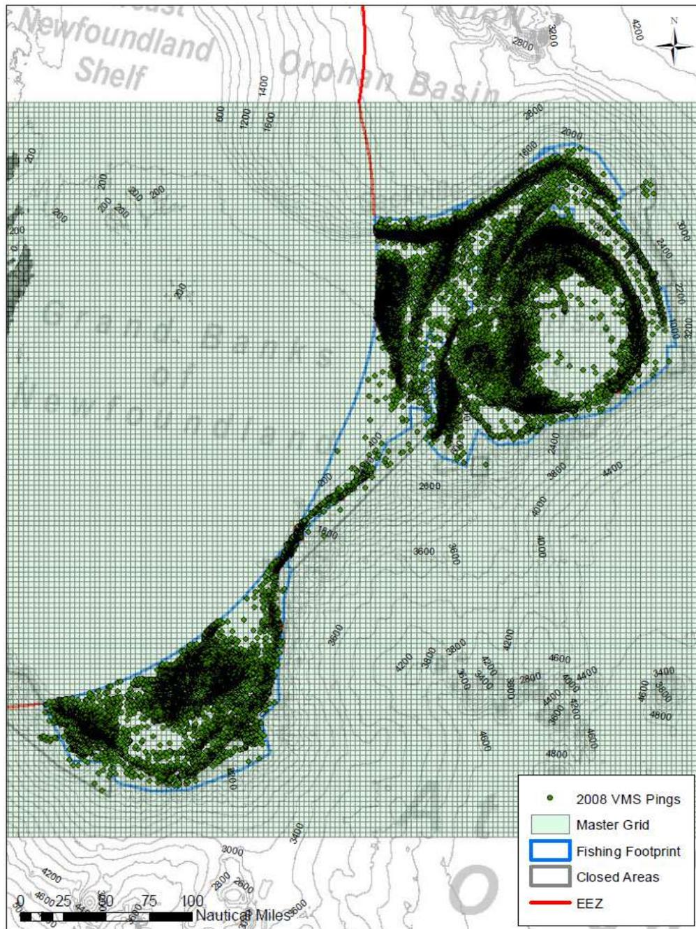
**Figure 4.2.2.1.1** VMS pings from 2008 with speeds between 0.5 and 5kts, clipped to the extent of the study area. The VMS ping counts within each grid cell were calculated to create a proxy surface of fishing intensity for each year where VMS data were available (2008 - 2011).
