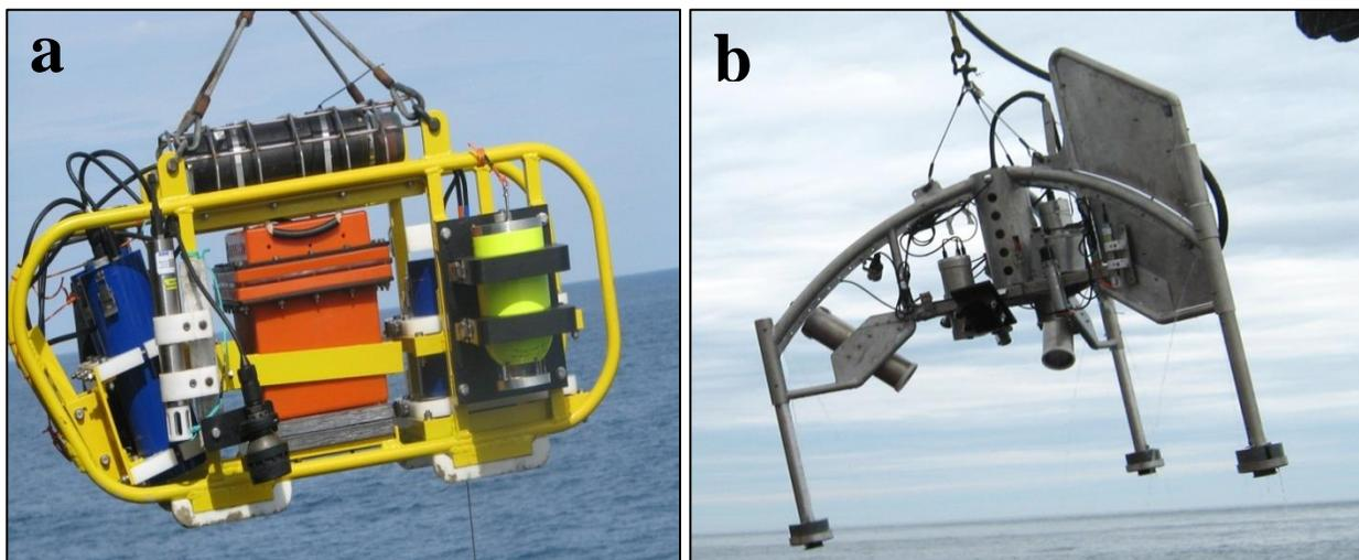
Figure 2. a) 4K camera (4KCam) and b) Campod camera systems used to collect benthic imagery during the 2009 *Hudson* cruise on the Flemish Cap.
