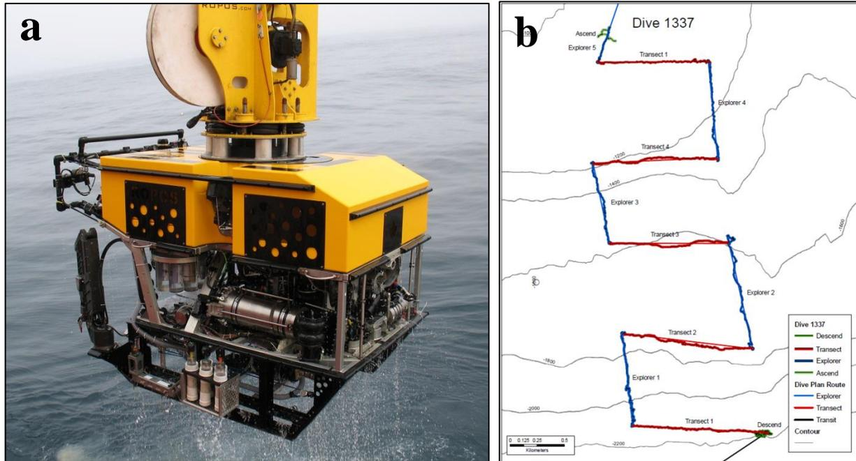
Figure 3. a) ROV ROPOS used to collect benthic imagery during the *Hudson* 2010 cruise to the Flemish Cap; b) example of a ROPOS transect consisting of both transect (red) and explorer (blue) modes.
