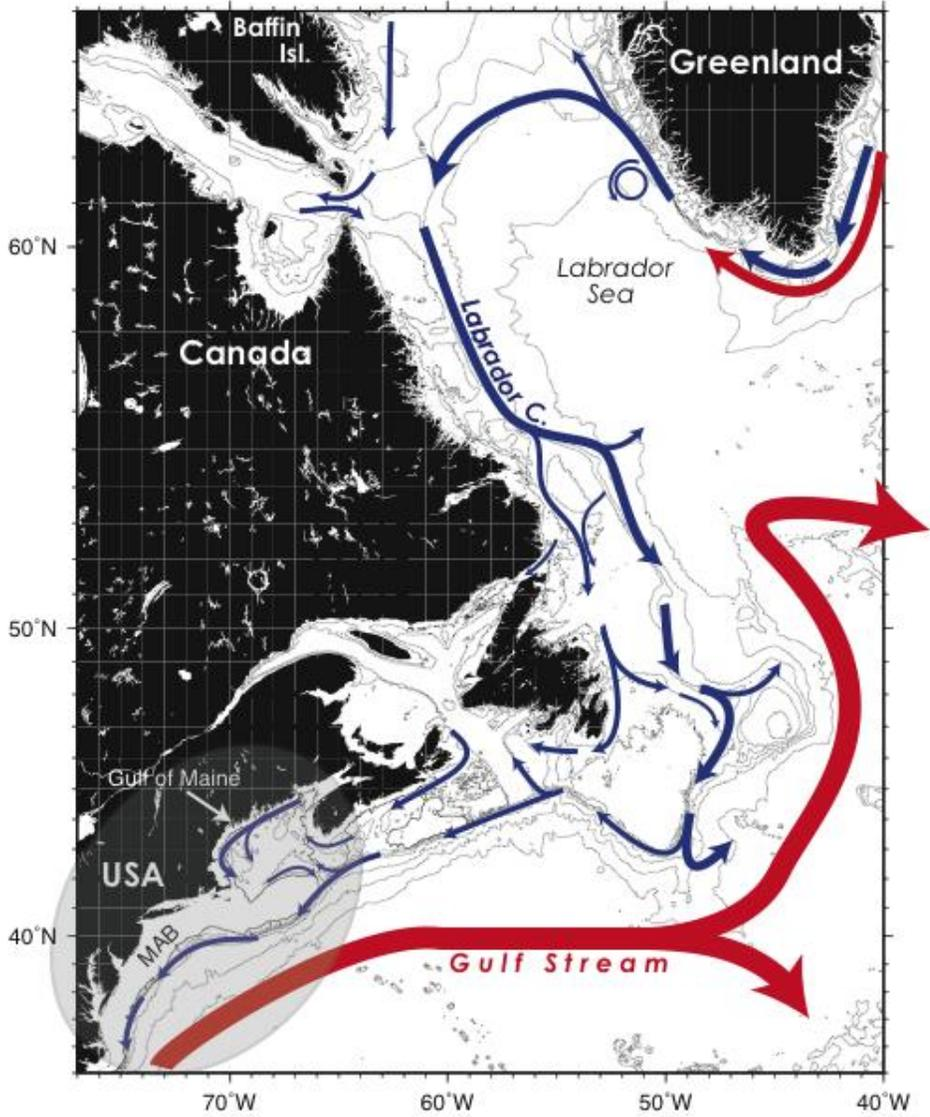
Fig. 1a. Circulation schematic of the western North Atlantic. The Northeast U.S. Shelf region is identified by the shaded oval. The 100, 200, 500, 1000, 2000, 3000 and 4000 meter isobaths are shown.
