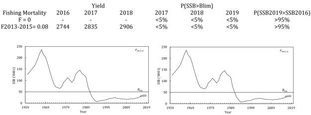
Fig. 11.13 American plaice in Div. 3LNO: Spawning stock biomass from projections along with  $10^{\text{th}}$  and  $90^{\text{th}}$  percentiles (dotted lines) for *F*=0 (left) and *F*<sub>2013-15</sub> (right).
