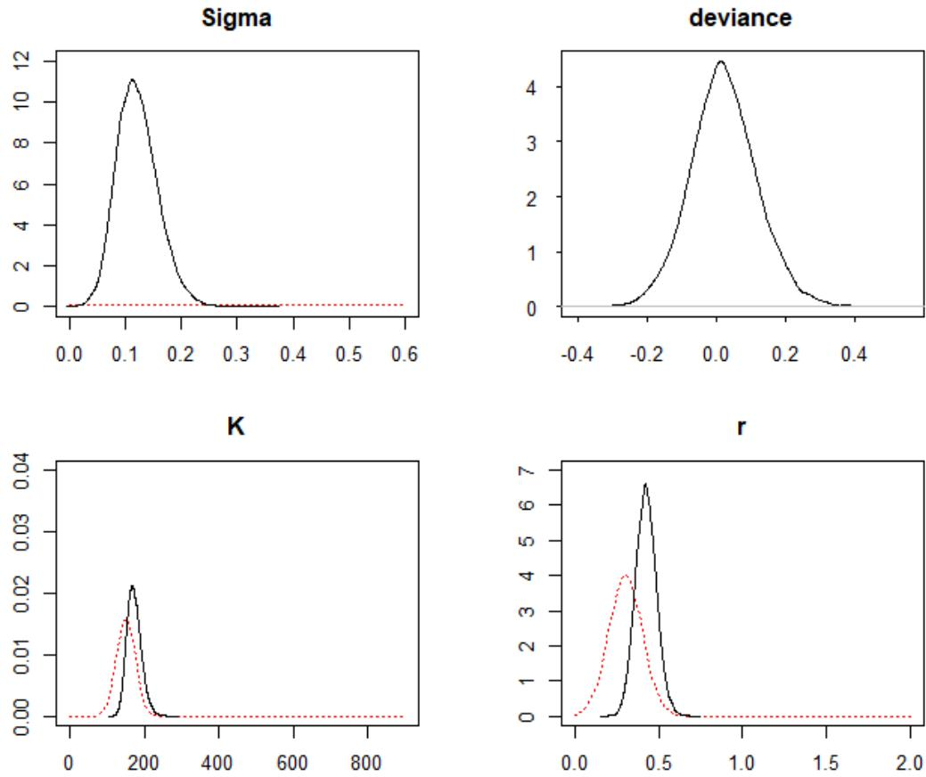
**Fig. 6.** Priors (red line) and posteriors (black line) for sigma (process error), deviance, carrying capacity (K) and intrinsic rate of growth (r) for the exploratory run of the Bayesian surplus production model.
